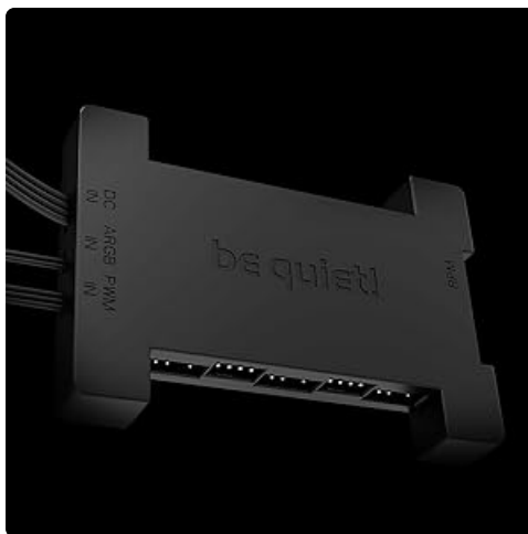
Image: The be quiet! ARGB-PWM-Hub, illustrating its various connection ports for ARGB components and PWM fans.
