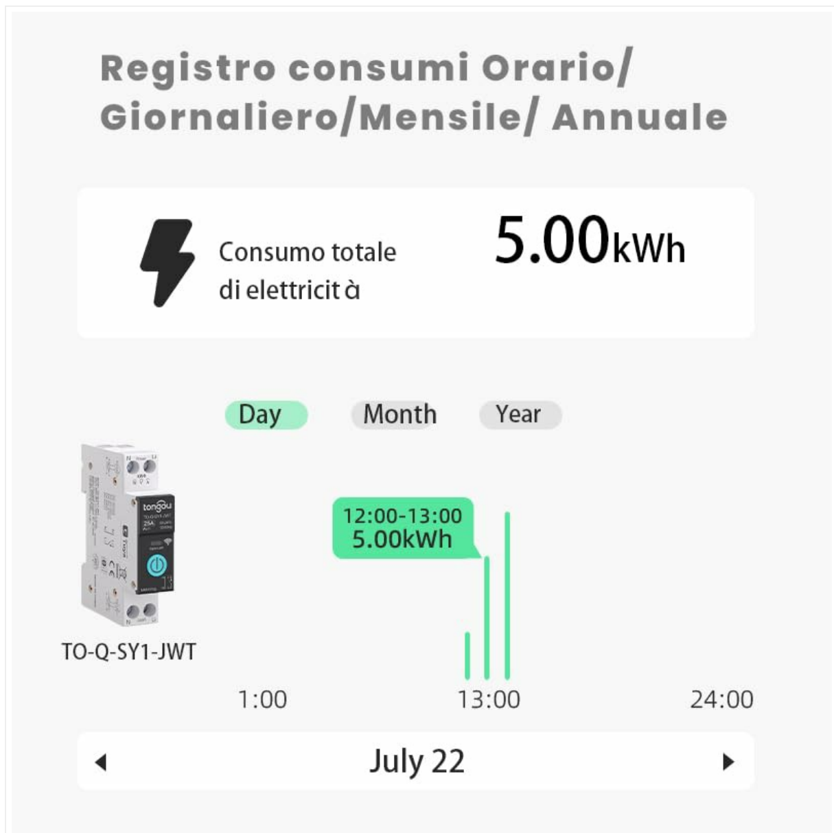
Figure 6.3: Example of the energy consumption log interface, displaying total electricity consumption over various time periods.
