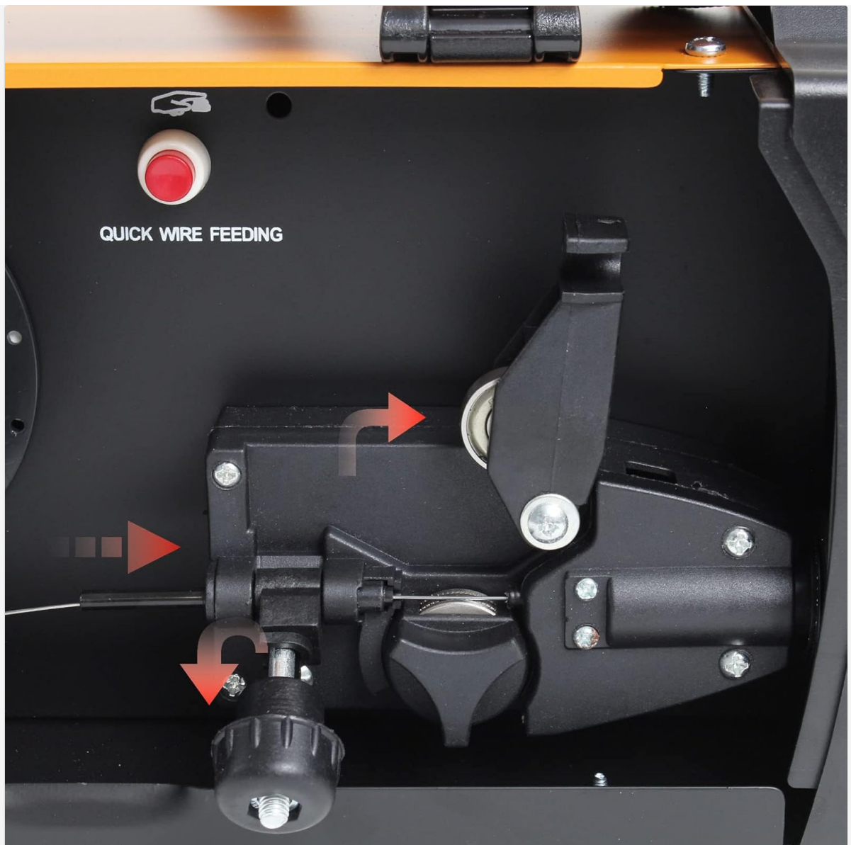
Image 5.3: Close-up of the wire feeding mechanism, with arrows indicating the direction of wire travel.
