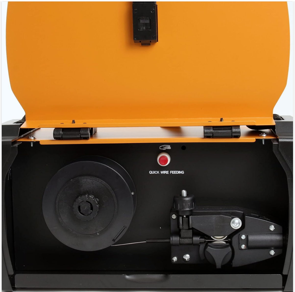
Image 5.2: Internal view of the welder, showing the wire spool mounted and the wire feeding mechanism. This image details the placement of the wire spool and the path the wire takes through the feeder.
