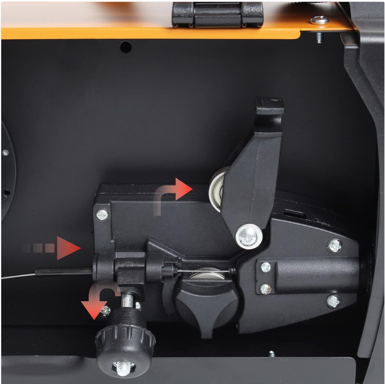
Figure 6: Wire feeding mechanism. The image shows the path of the welding wire through the drive rollers and guide tubes, with red arrows indicating the correct direction of wire travel.
