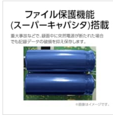
Image: A super capacitor, which provides file protection by preventing data corruption during sudden power interruptions.
