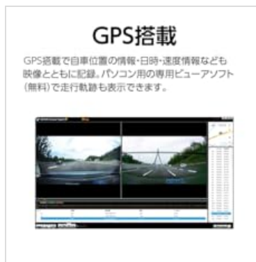
Image: Screenshot of the PC viewer software, displaying synchronized video footage from both cameras with GPS data, including location on a map, speed, and time.
