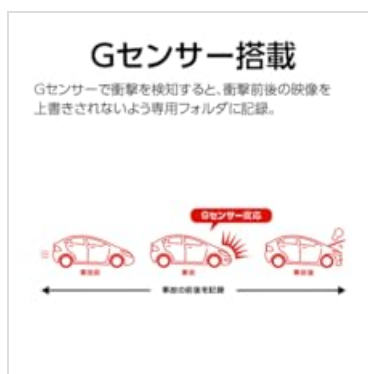
Image: Diagram illustrating the G-sensor's function, showing how it detects an impact and saves the surrounding video footage.
