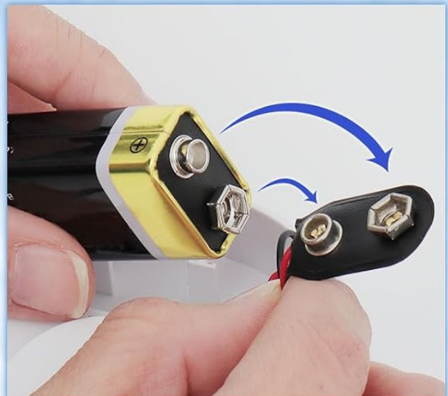
2. Confirm the positive/negative poles
