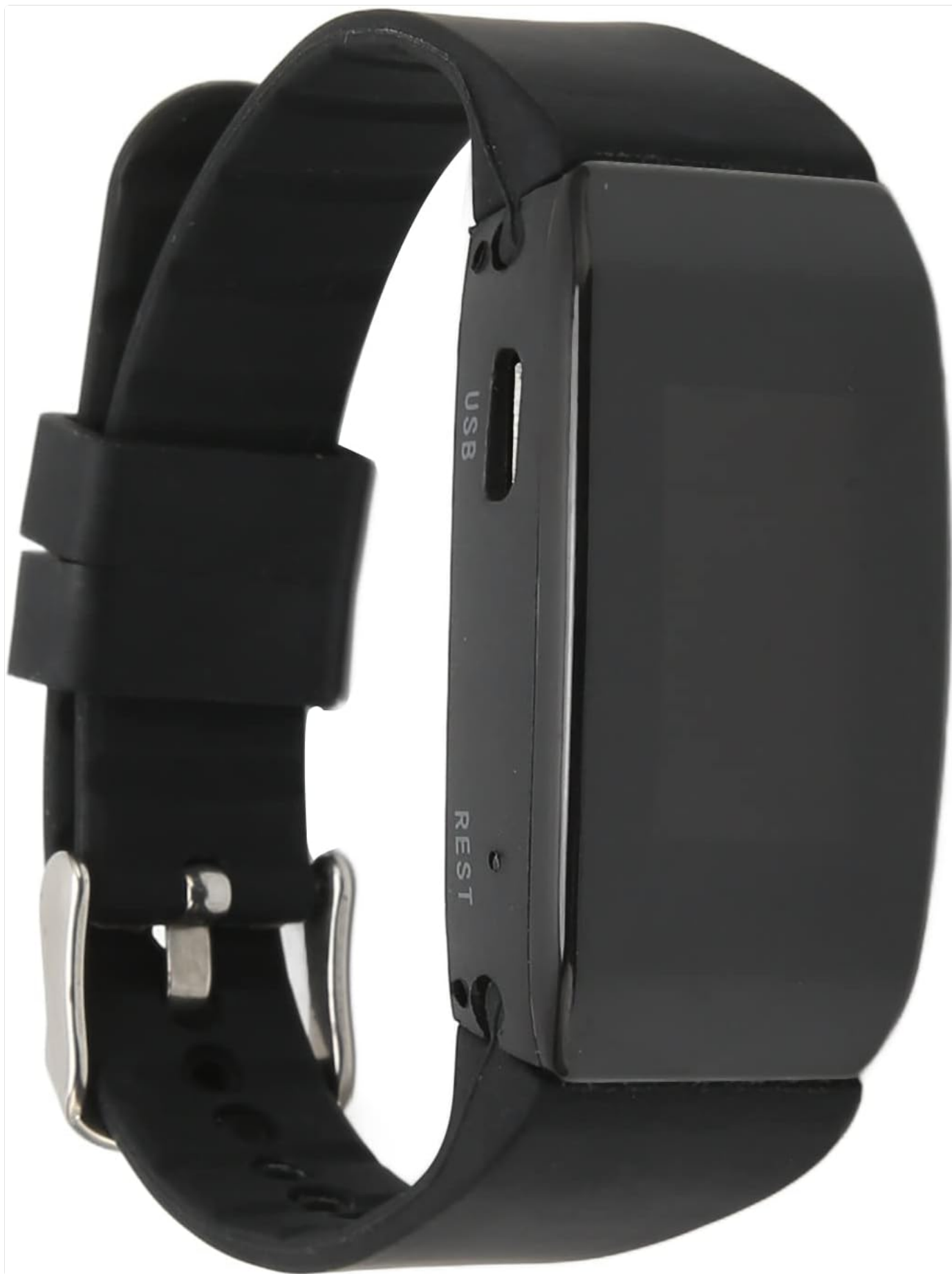
Figure 2.2: Side view of the watch, highlighting the USB port for charging and data transfer.
