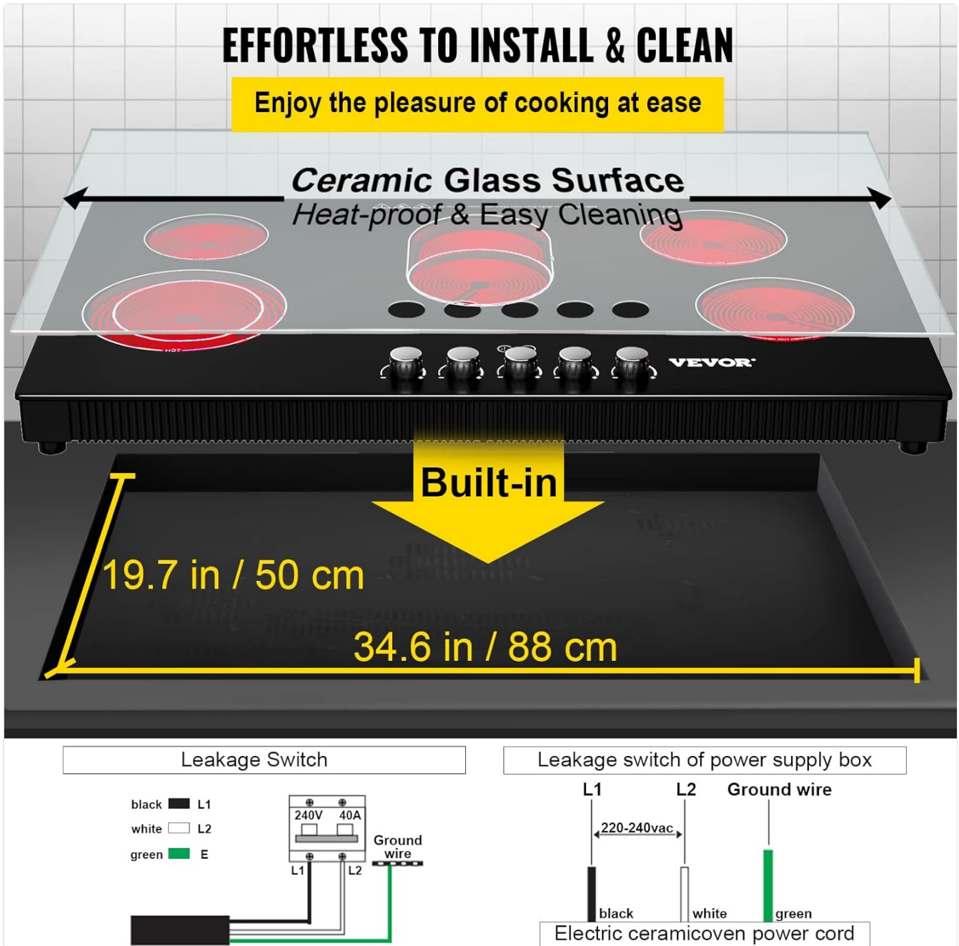
Image: Diagram showing the built-in installation process with cutout dimensions (34.6 in / 88 cm width, 19.7 in / 50 cm depth) and a detailed electrical wiring diagram for 220-240VAC connection, including L1, L2, and Ground wire connections.
