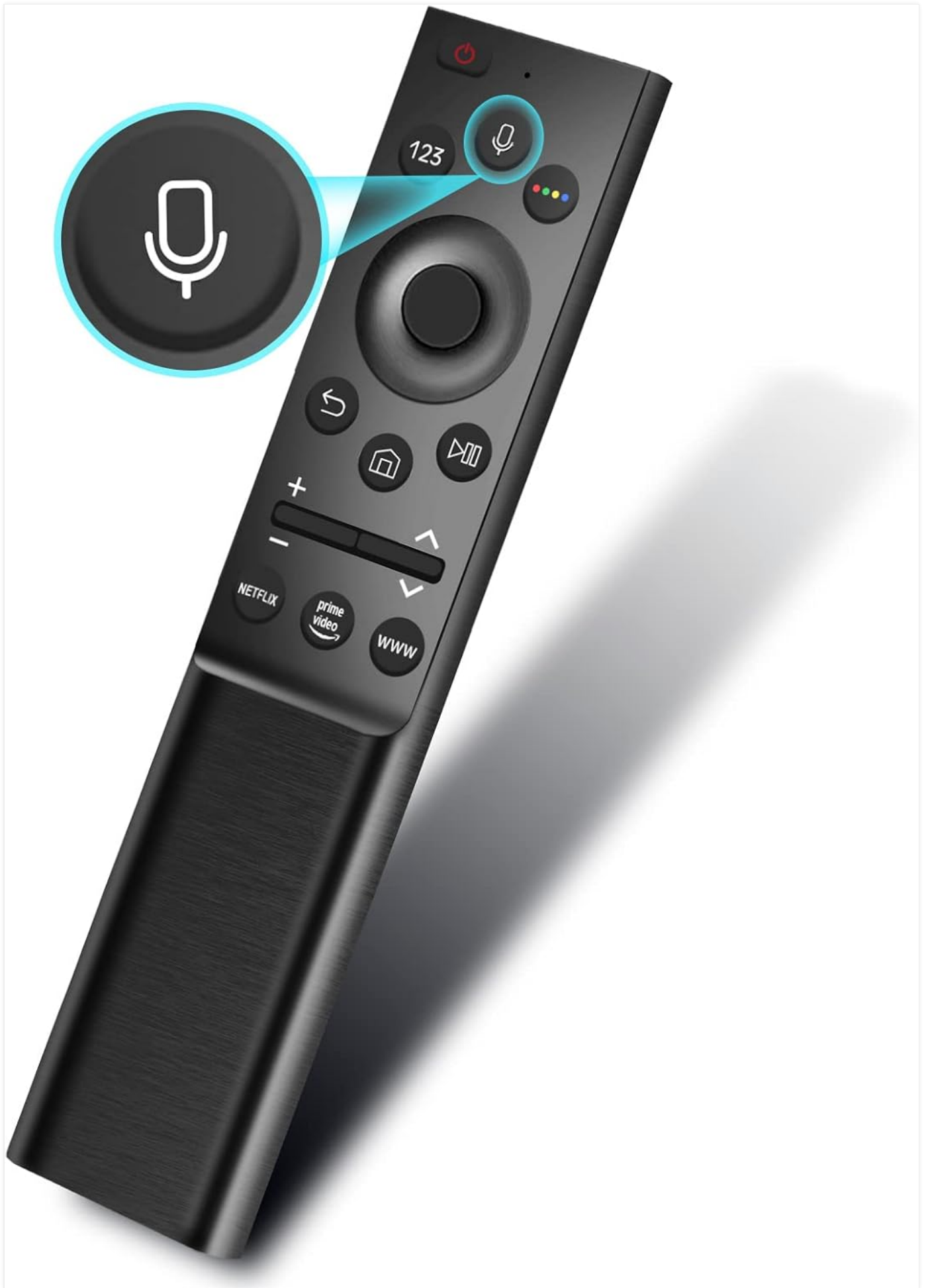
Figure 2: Remote control layout with microphone button highlighted. This button activates voice control features on compatible TVs.
