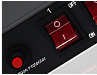
Figure 4.1: Individual ON/OFF Switch
