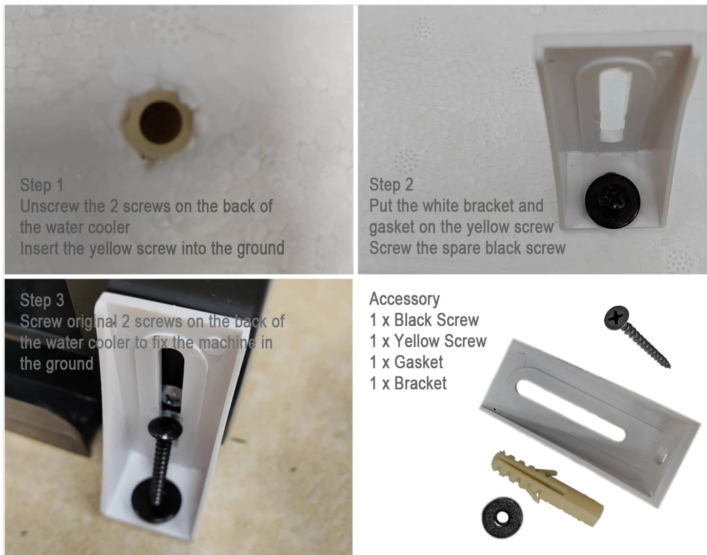
Image 3.1: Components for securing the water cooler, including a bracket, screws, and gasket, along with step-by-step instructions for installation.
