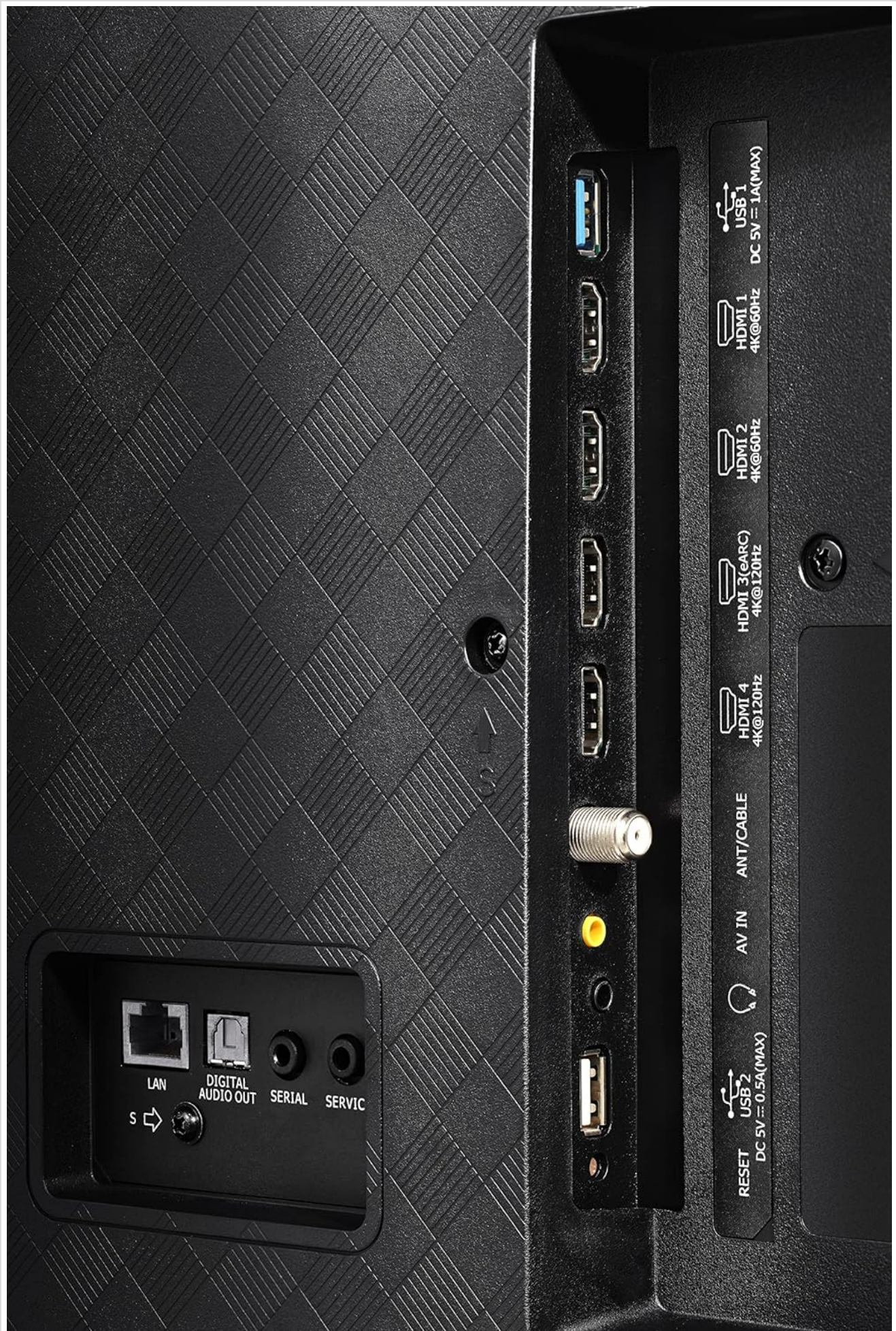
Image: Close-up of the rear panel of the Hisense U7H TV, showing various input ports including HDMI, USB, LAN, and Digital Audio Out.
