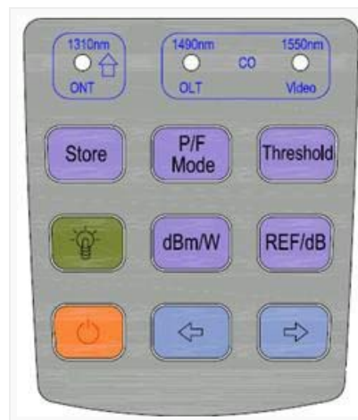
Figure 1: Deviser EP310 PON Power Meter Control Panel. This image displays the button layout and their primary functions, including wavelength selection (1310nm, 1490nm, 1550nm), Store, P/F Mode, Threshold, backlight, dBm/W, REF/dB, Power On/Off, and navigation buttons.
