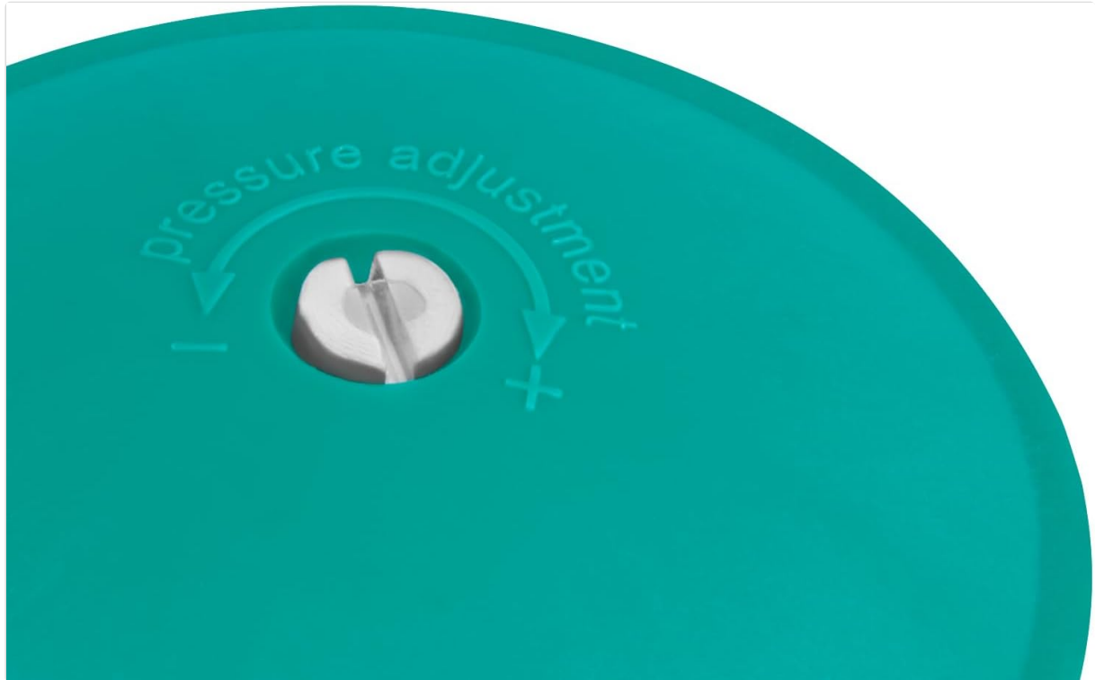
Figure 5.1: Pressure adjustment screw on the pressure switch. Adjusting this screw can modify the cut-in pressure of the pump.
