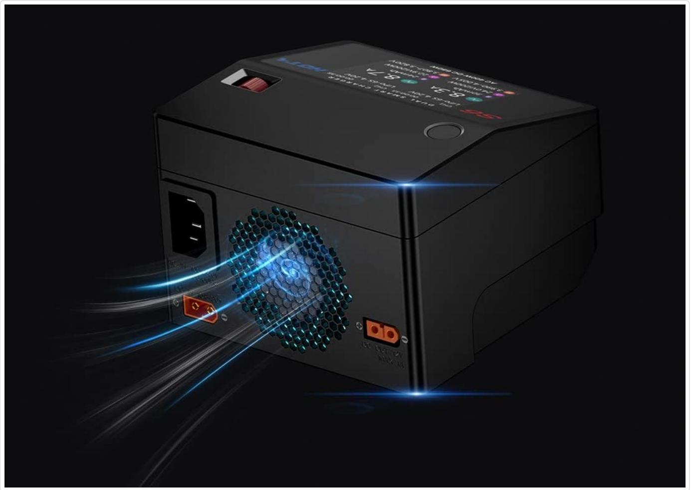
Figure 4: Illustration of the cooling airflow through the rear fan of the HOTA S6 charger, demonstrating its active cooling system for stable operation.
