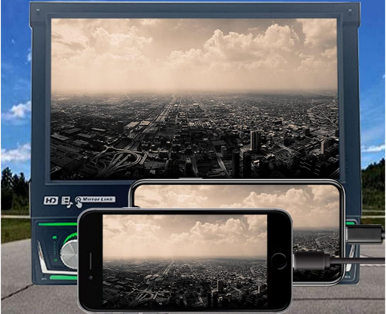
Image: The car stereo screen mirroring a smartphone, demonstrating the Mirror Link feature.
