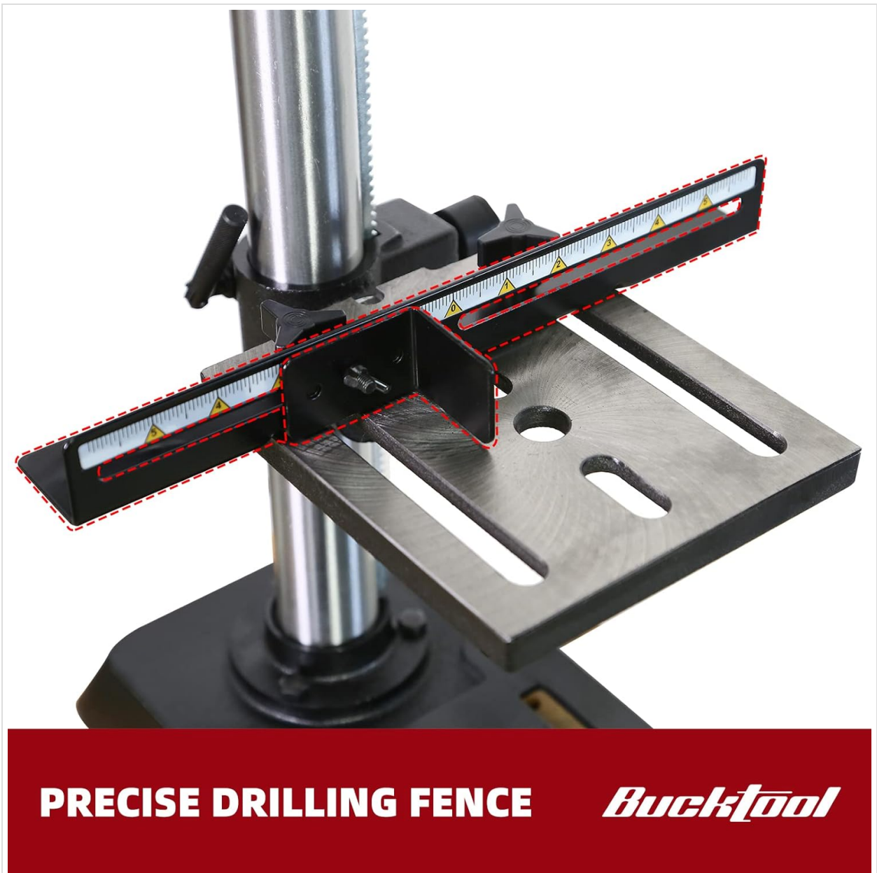
Figure 3.3: The drill press table equipped with the precise drilling fence, designed to aid in accurate positioning and support of the workpiece.
