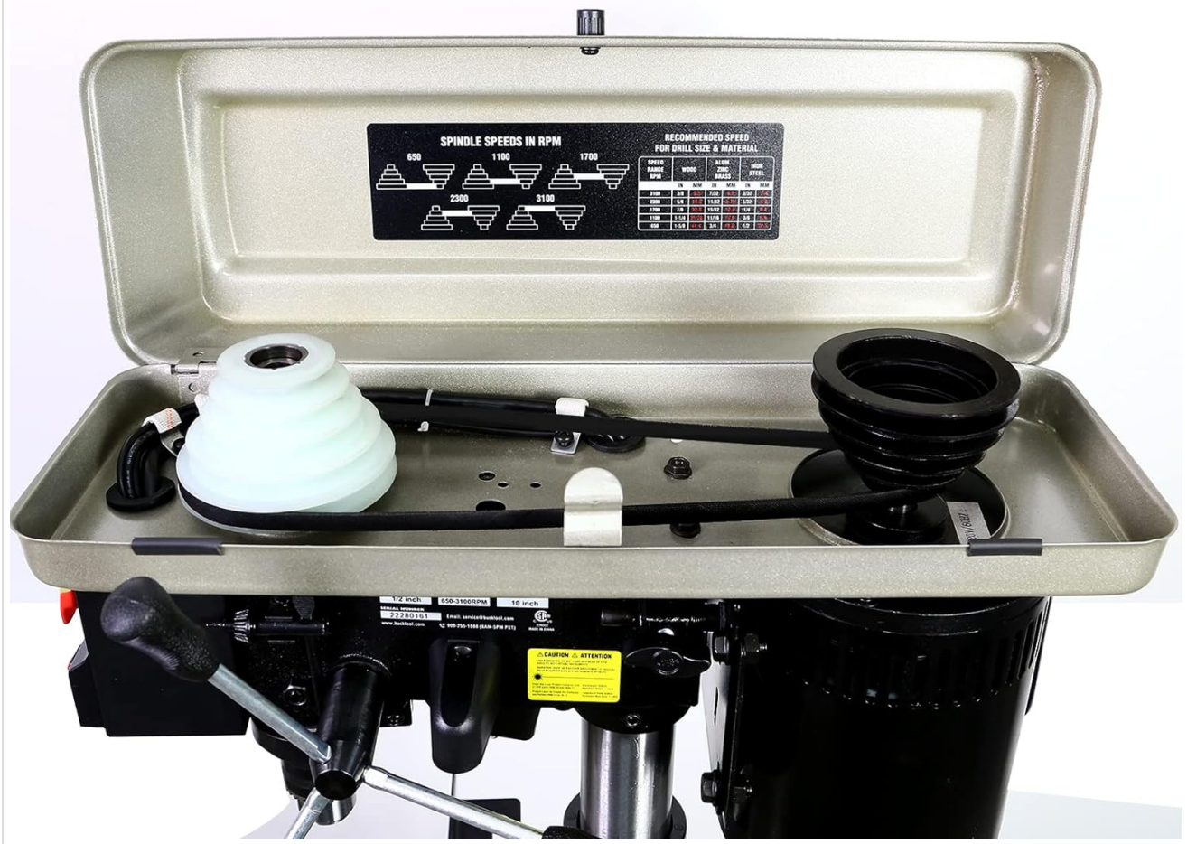
Figure 3.2: View inside the drill press head, illustrating the belt and pulley system used to adjust the spindle speed. A speed chart is typically located on the inside cover for reference.
