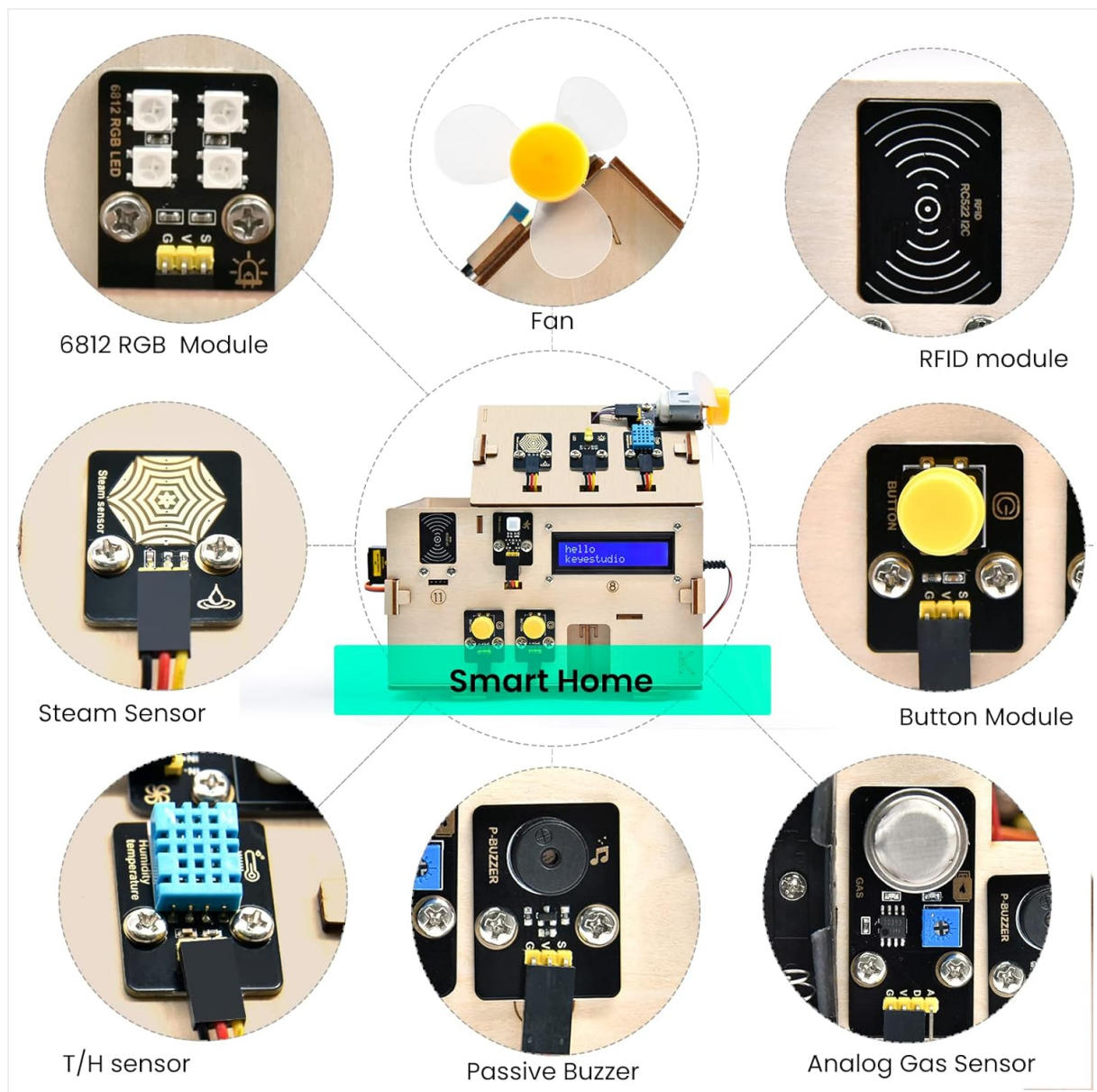
Figure 2: Diagram illustrating various sensor and control modules included in the kit.
