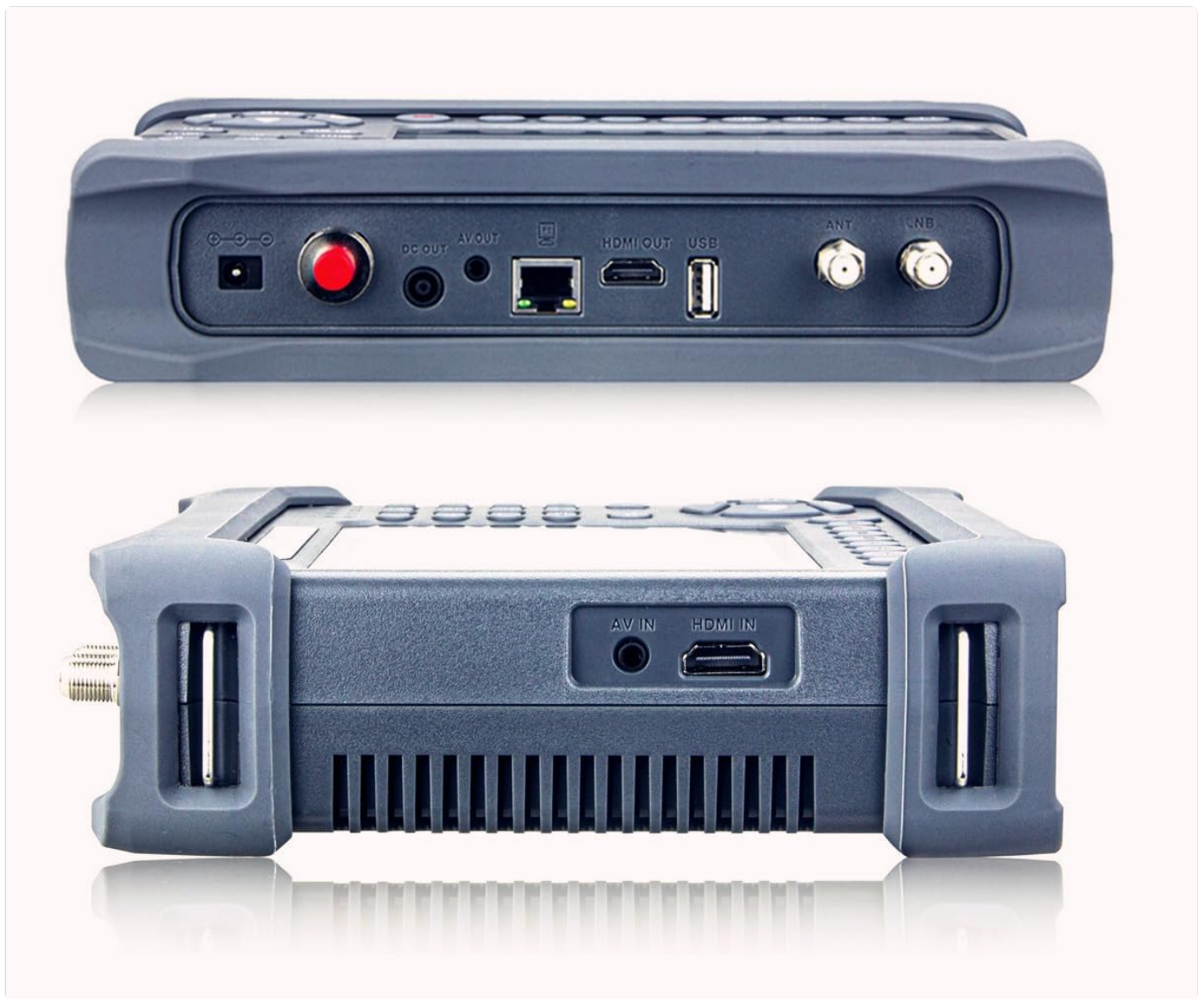
Figure 2.2: Top and side views illustrating connectivity ports.
