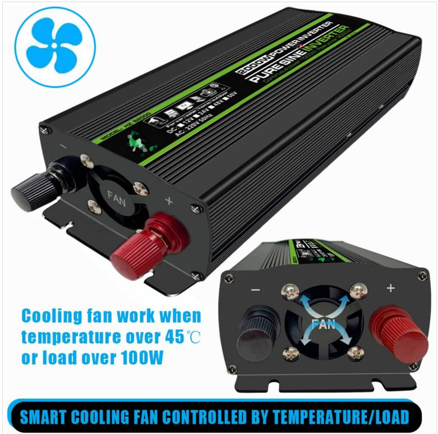
Image 5.1: Illustration of the FONOBO Power Inverter's smart cooling fan. This image shows the fan's location and explains that it operates when the temperature exceeds 45°C or the load exceeds 100W.
