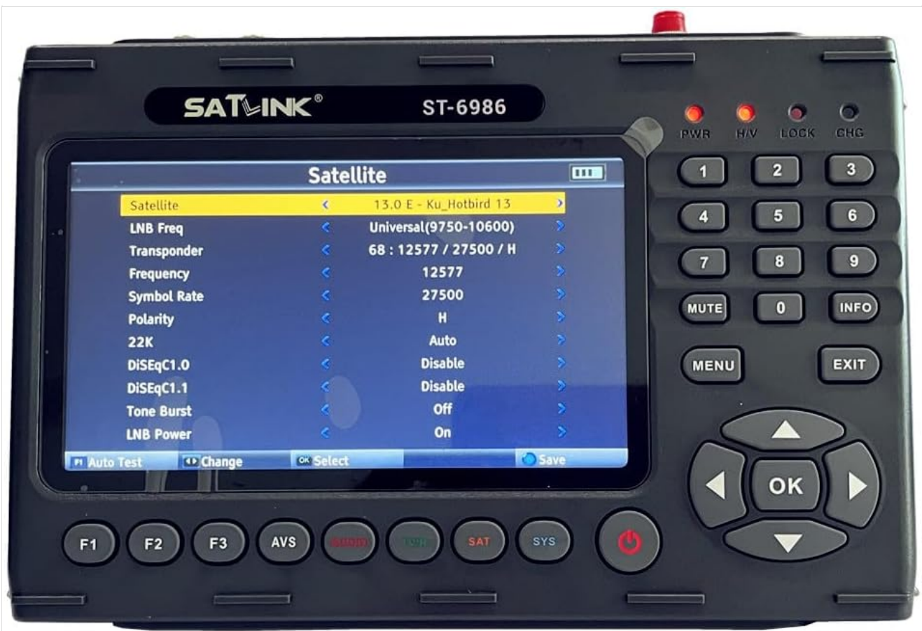
Figure 5.1: Satellite settings screen for configuring LNB, transponder, and other parameters.
