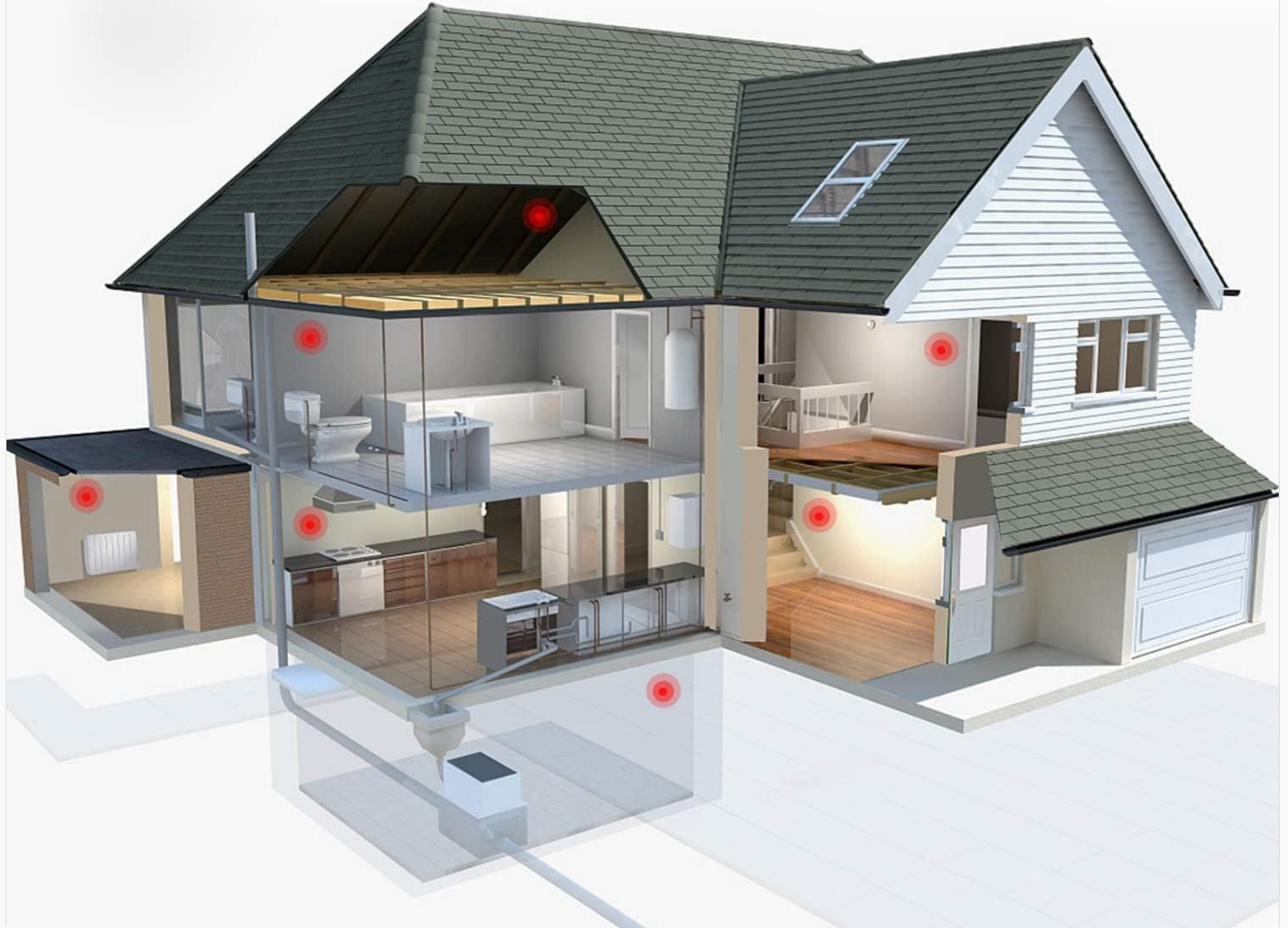
Image: A cutaway diagram of a house illustrating optimal placement of interconnected smoke alarms on different floors and areas.
