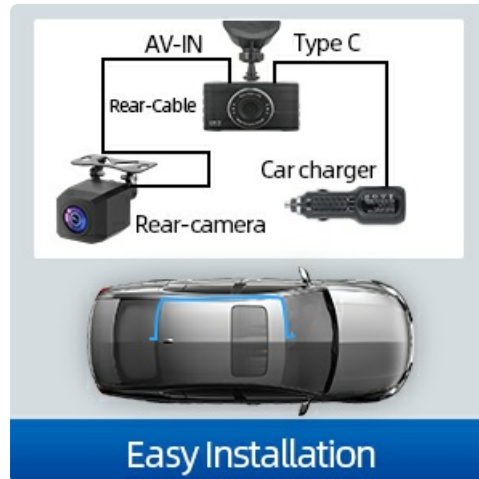
Image 4.2: Simplified diagram of the dash cam and rear camera installation.
