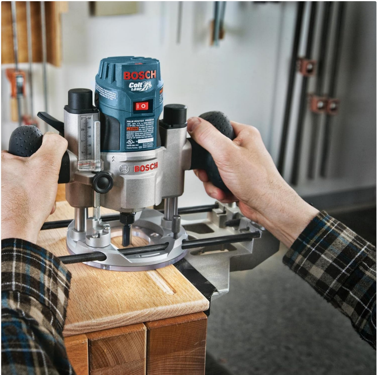
Image 5.1: A fixed-base router in operation, demonstrating a typical routing application on a wooden surface.
