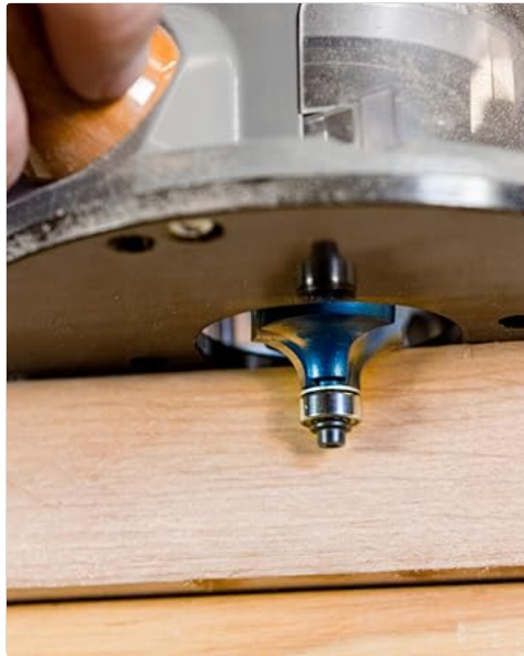
Image 4.1: Proper insertion of a router bit into the collet, ensuring a secure fit.
