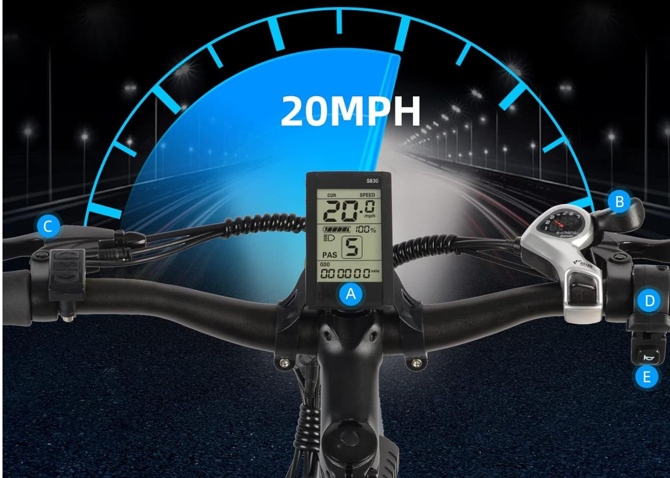
This image provides a detailed view of the bike's handlebars, highlighting the 5-level LCD display, Shimano 7-speed shifter, dual disc brake levers, throttle, and horn button, all designed for fingertip control.
