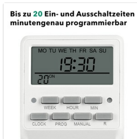
Image: The timer display showing a programmed ON time, illustrating the capacity for 20 programs.
