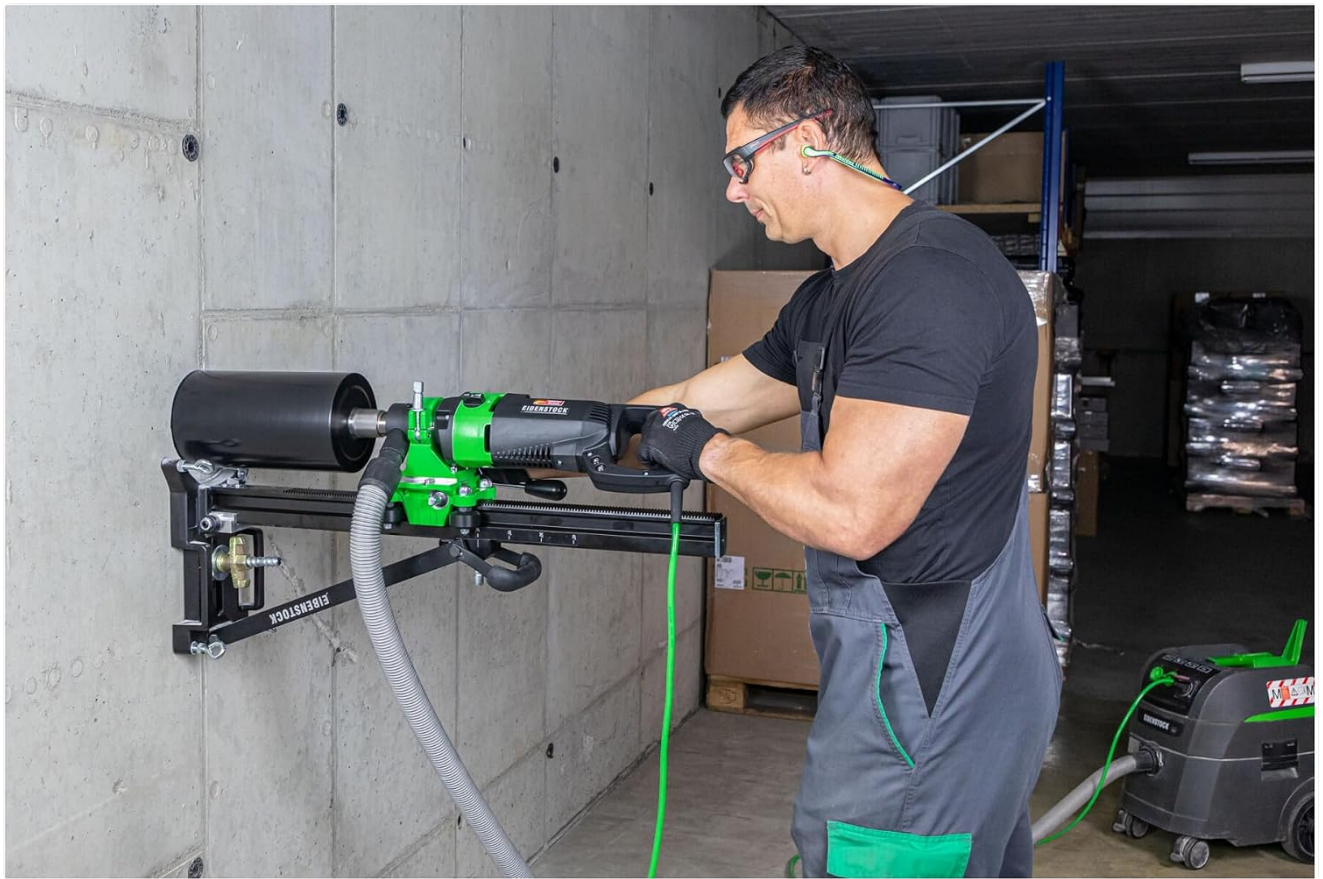
Figure 3: An operator demonstrating the use of the Eibenstock ESD 162 with a drill stand for dry core drilling. Note the dust extraction hose connected for efficient dust management.
