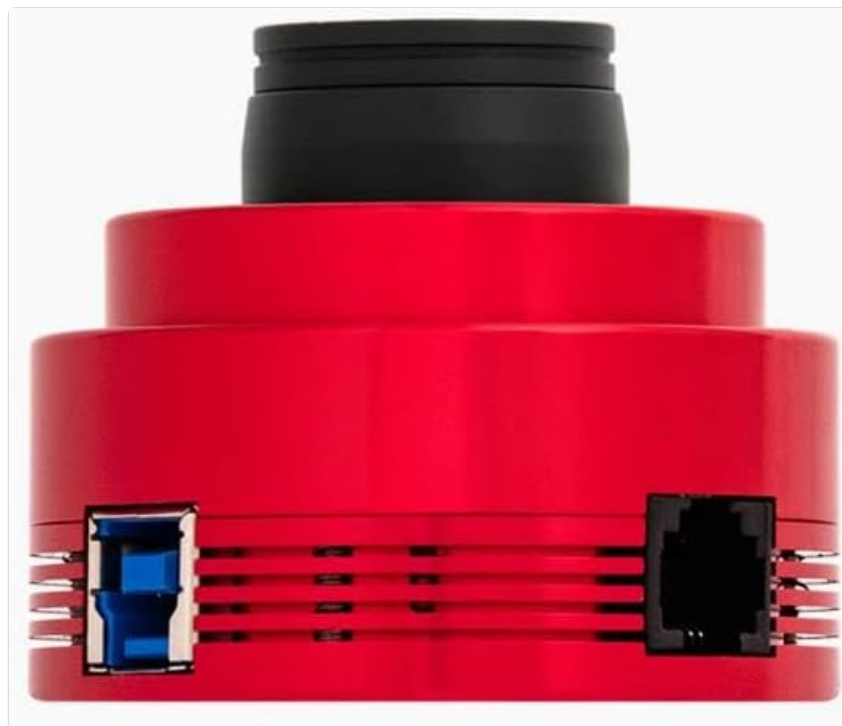
Figure 3.1: Side view of the camera showing USB3.0 and ST4 ports.
