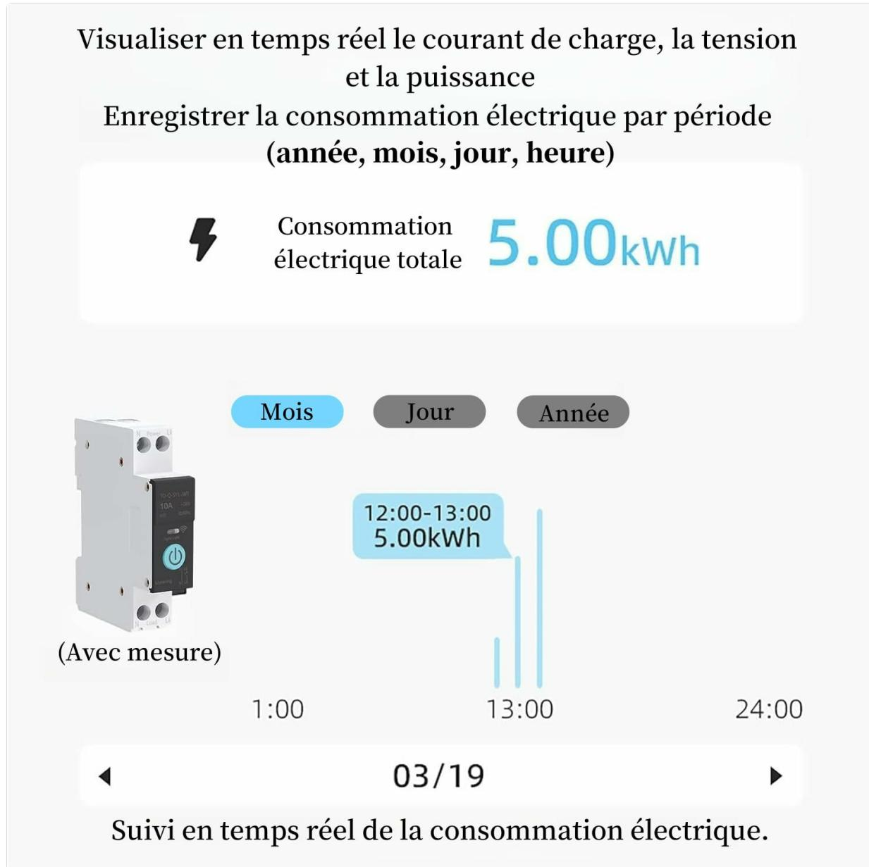
Image: Real-time energy consumption monitoring interface in the app.
