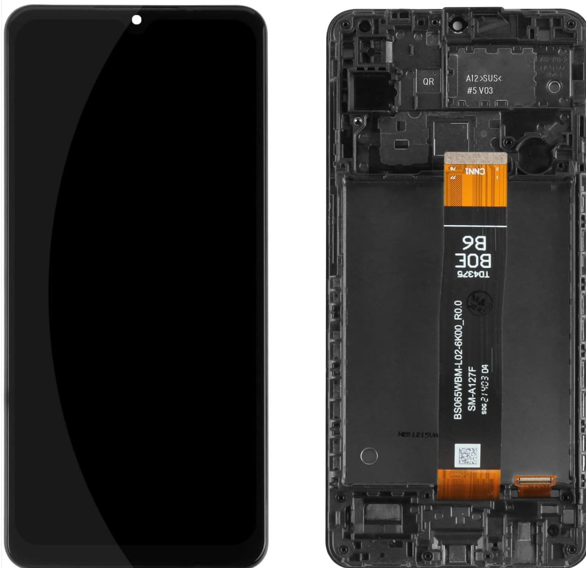
Image 5.1: The new LCD screen with its integrated frame, ready for installation. This design simplifies the replacement process compared to frameless screens.
