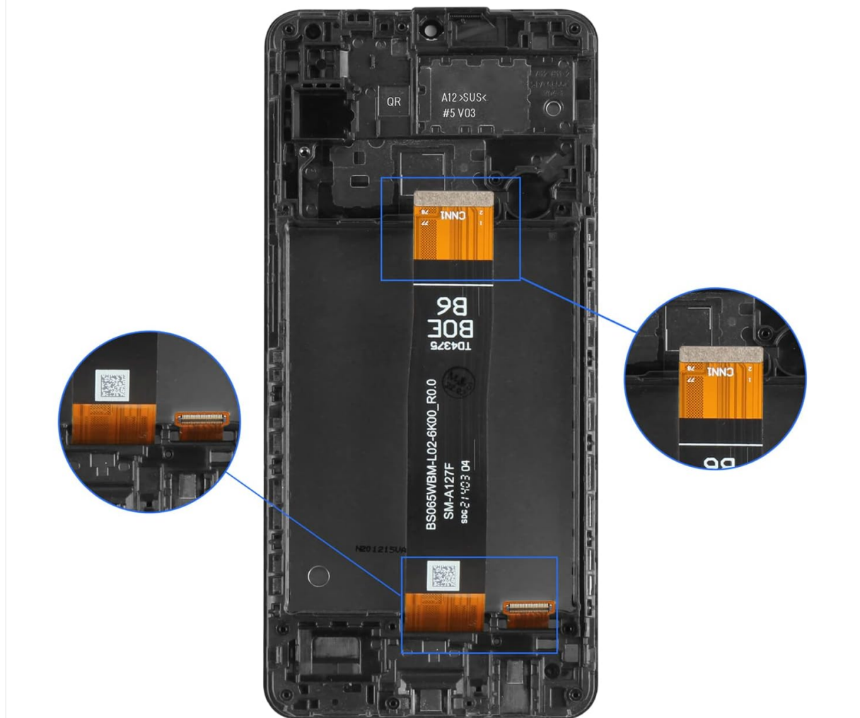
Image 5.2: Close-up view of the flex cable connections on the screen assembly, highlighting the points where it connects to the phone's motherboard.
