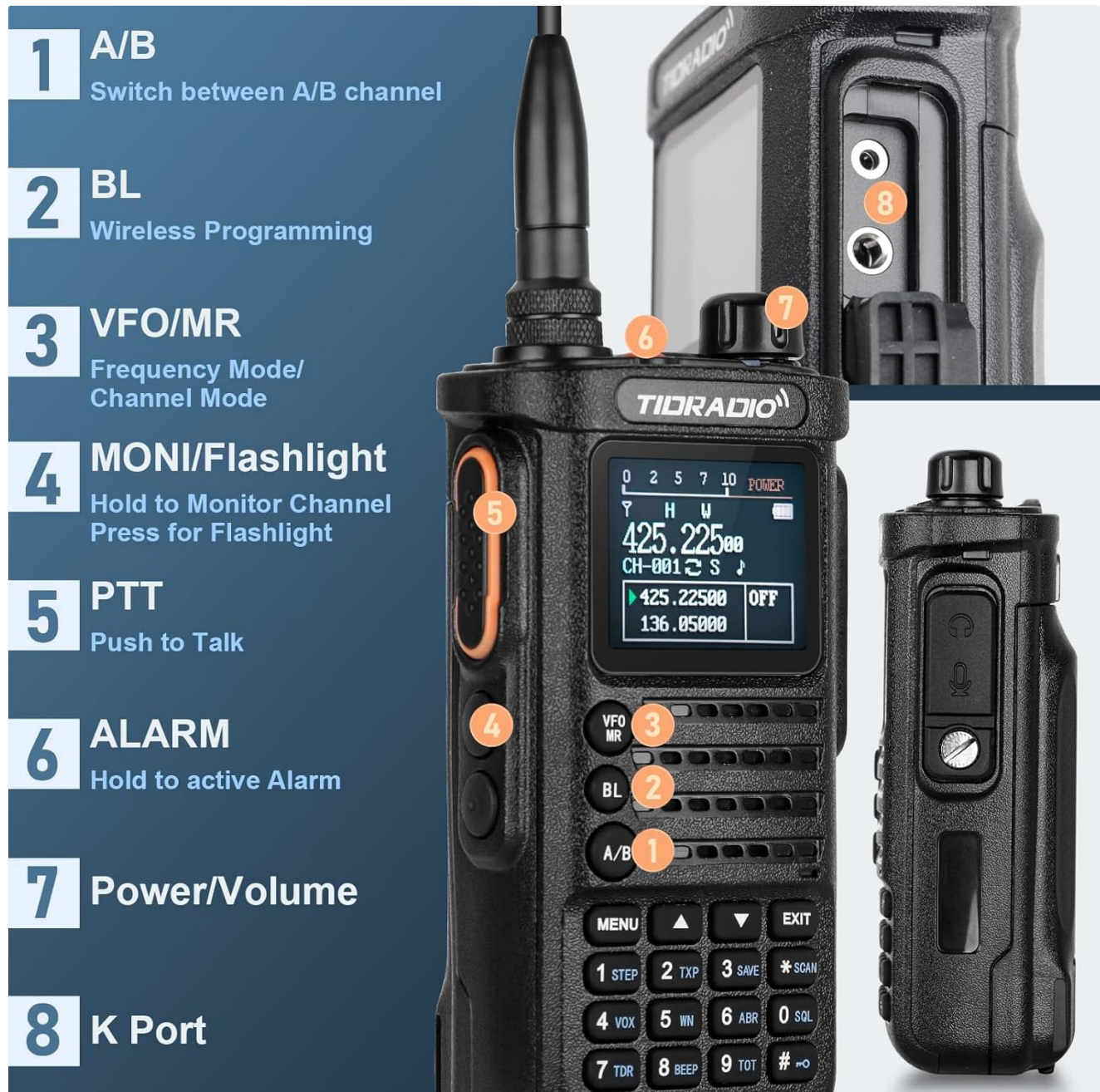
Image: A detailed diagram of the TD-H8 radio, labeling its various buttons and ports.
