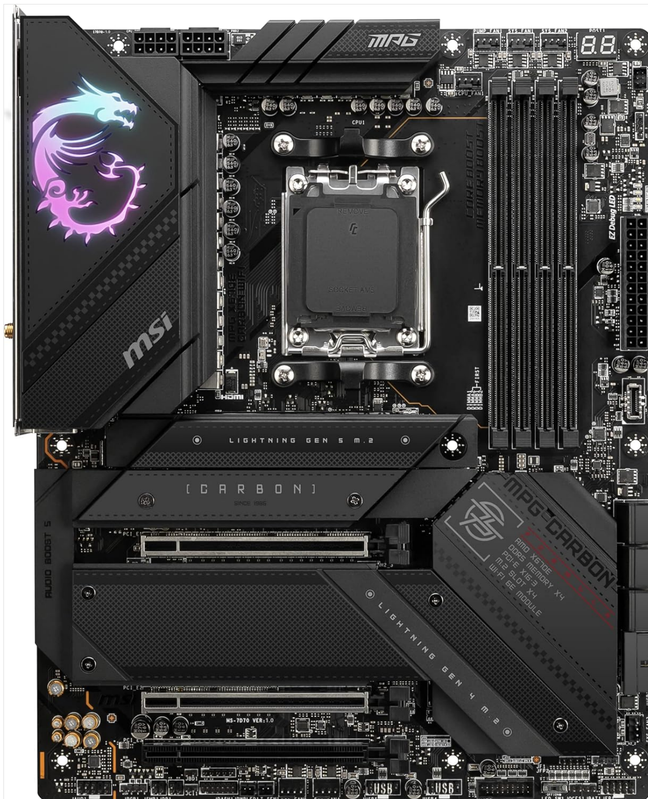
Figure 4.1: Top-down view of the MSI MPG X670E Carbon WiFi Motherboard. This image displays the CPU socket (AM5), four
