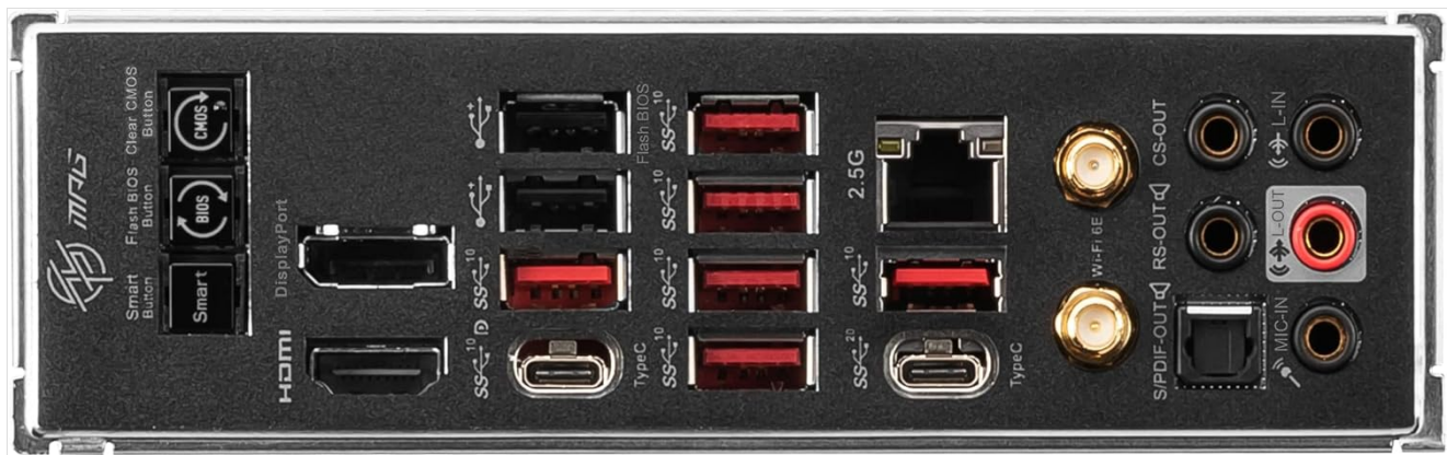
Figure 4.3: Rear I/O Panel of the MSI MPG X670E Carbon WiFi Motherboard. This panel includes USB 3.2 Gen 2 ports (Type-A and Type-C), HDMI, DisplayPort, 2.5Gbps LAN port, Wi-Fi 6E antenna connectors, audio jacks, and the Flash BIOS Button with Clear CMOS button.
