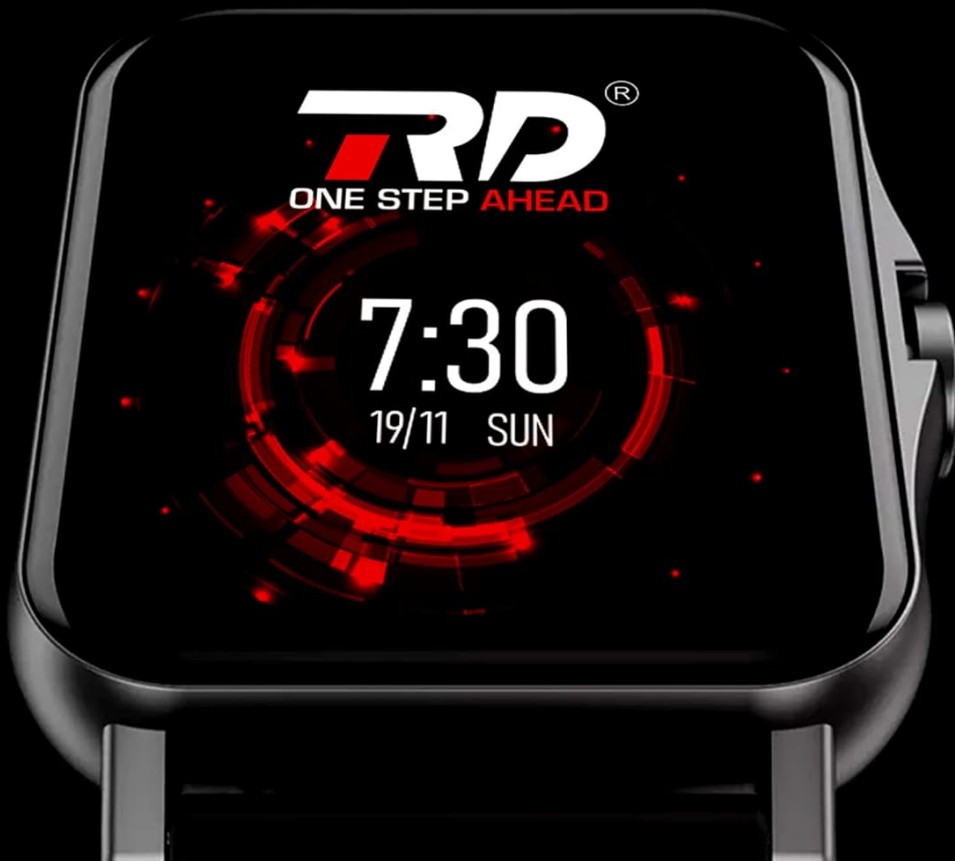
Figure 3.2: The 1.69-inch full-touch display with 240x280 pixel resolution.
