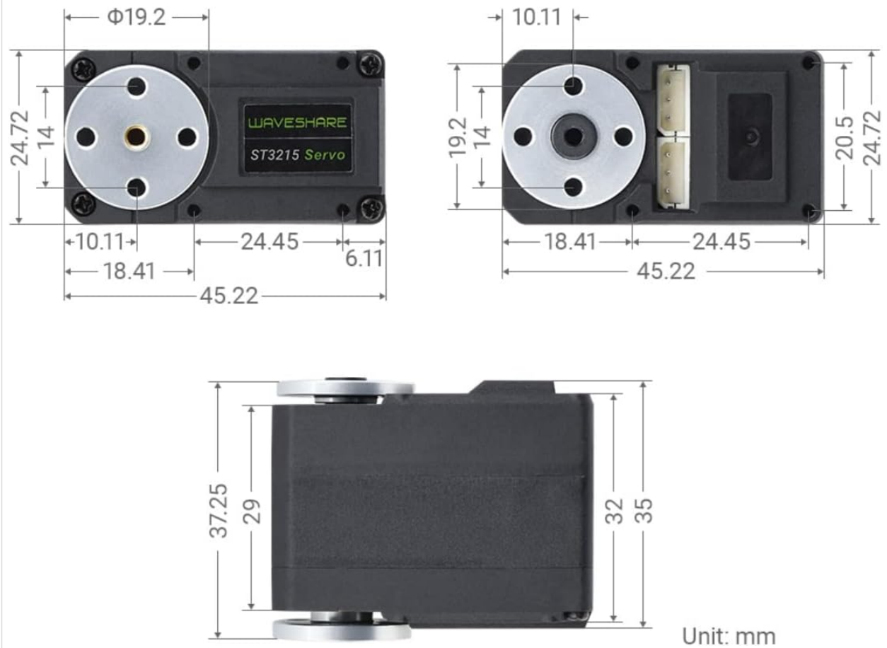
Figure 5.1: Outline dimensions of the ST3215 servo motor, with measurements in millimeters.
