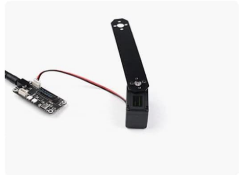
Figure 4.2: Step-by-step guide for calibrating the middle position of the ST3215 servo using a control interface.
