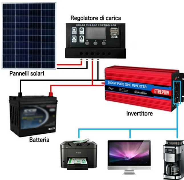
Figure 7: Connection diagrams for the inverter, including options for solar panel integration or direct battery connection.
