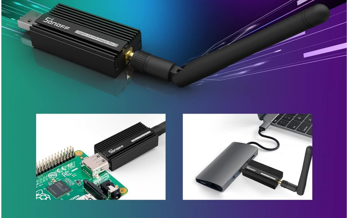
Image 2.1: The Dongle Plus-E connected to a Raspberry Pi and a laptop, illustrating its use as a universal Zigbee USB stick.
