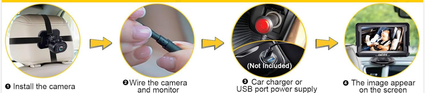
Figure 4.1: Step-by-step guide for quick installation.
