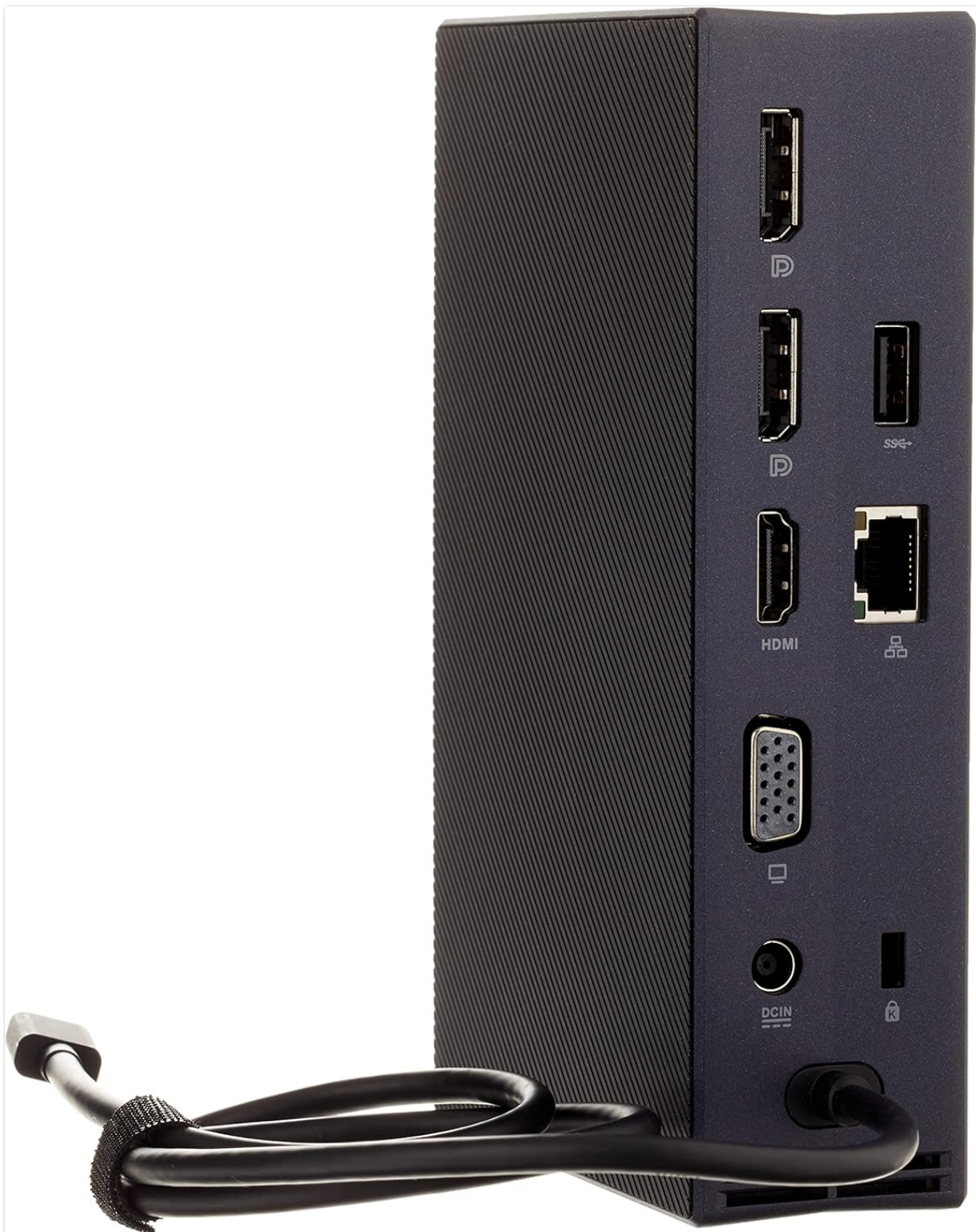
Figure 3.3: Rear view of the ASUS SIMPRO Dock 2. This image illustrates the connectivity options on the back of the dock, including various display outputs, Ethernet, USB-A, and the power input.
