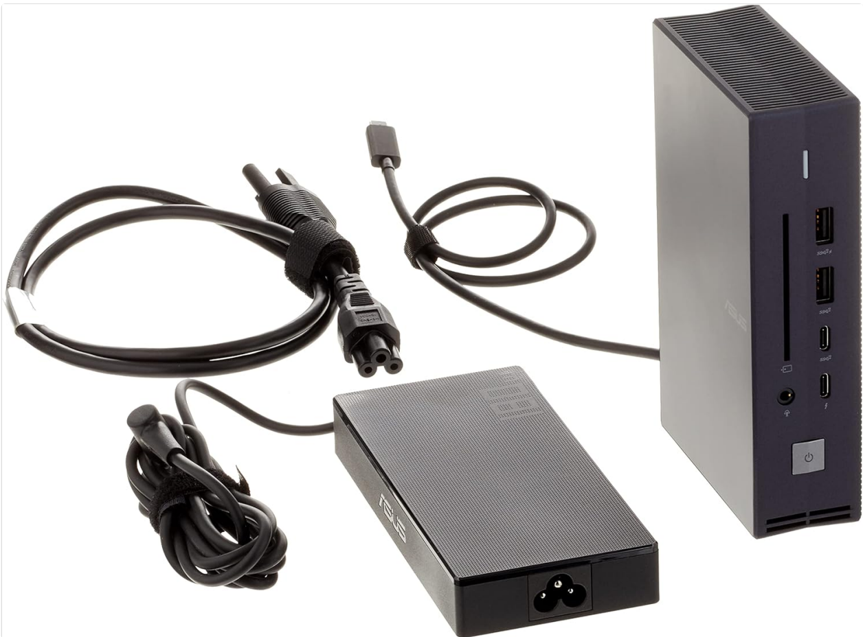
Figure 2.1: ASUS SIMPRO Dock 2 with included power adapter and Thunderbolt cable. This image shows the main docking unit, its power supply, and the Thunderbolt connection cable.
