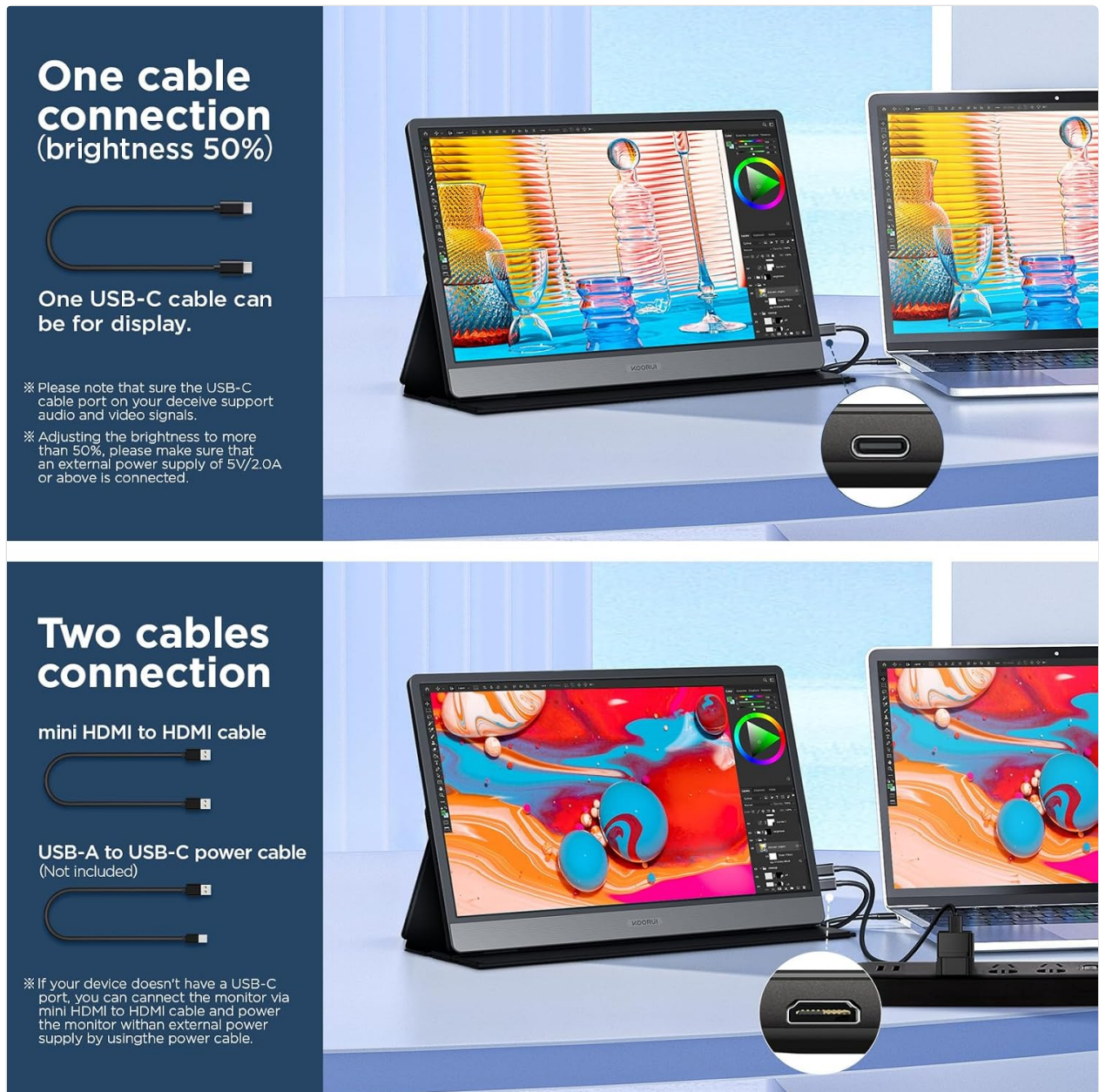
Figure 4.1: Single vs. Dual Cable Connection
