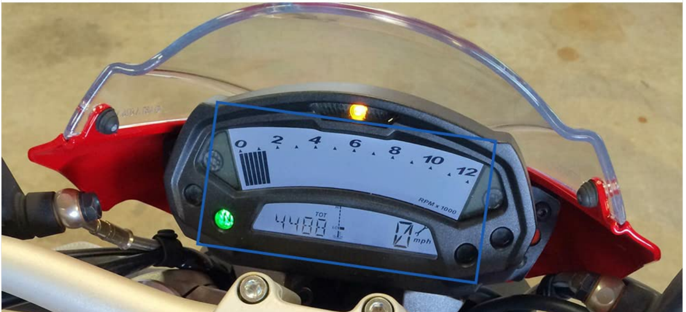
Figure 4: The A-BENET display shown in an application scenario for a Ducati Monster 796 instrument cluster (2010-2014 model years). This image highlights the display's fit and appearance within the cluster.
