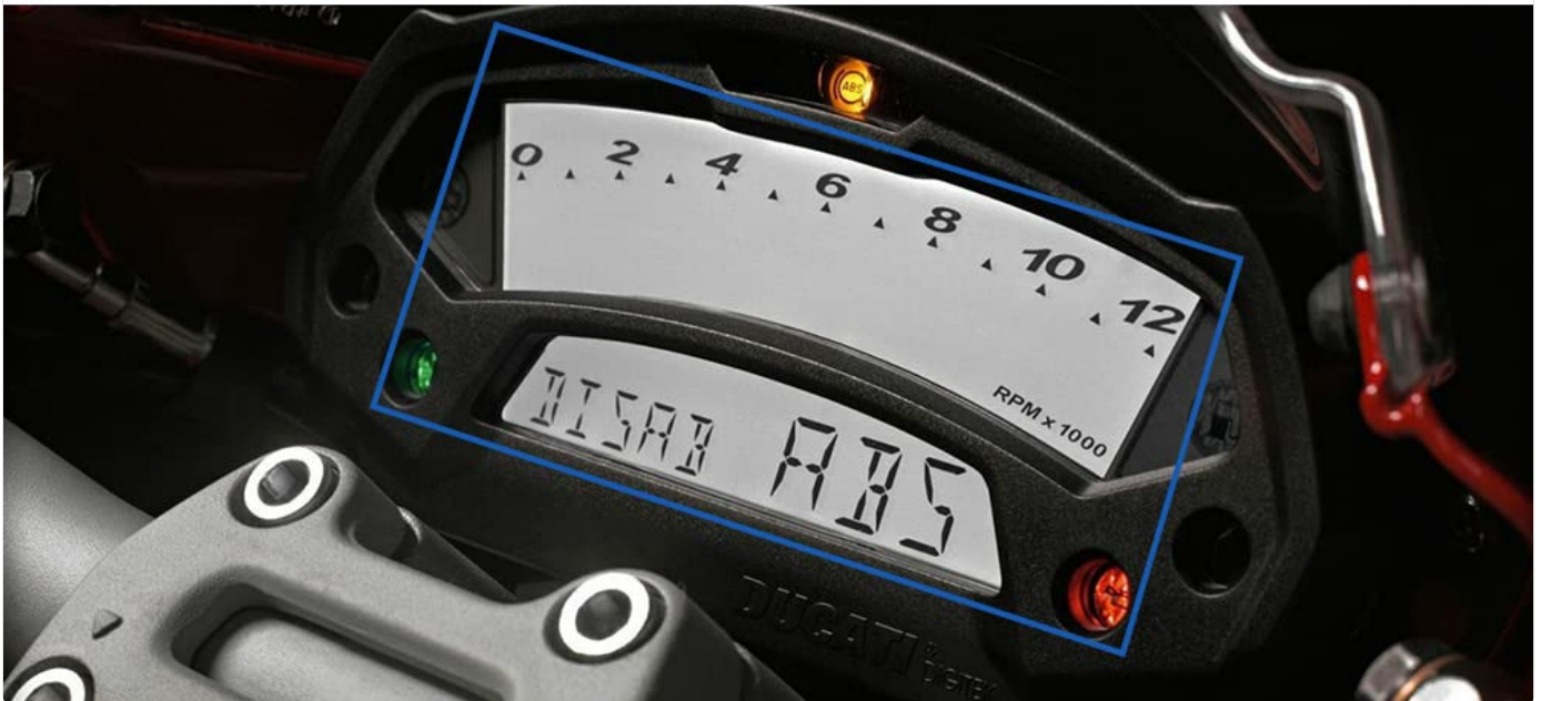
Figure 3: The A-BENET display shown in an application scenario for a Ducati Monster 1100 Evo instrument cluster (2011-2013 model years). Note the clear white backlight and digital readouts.
