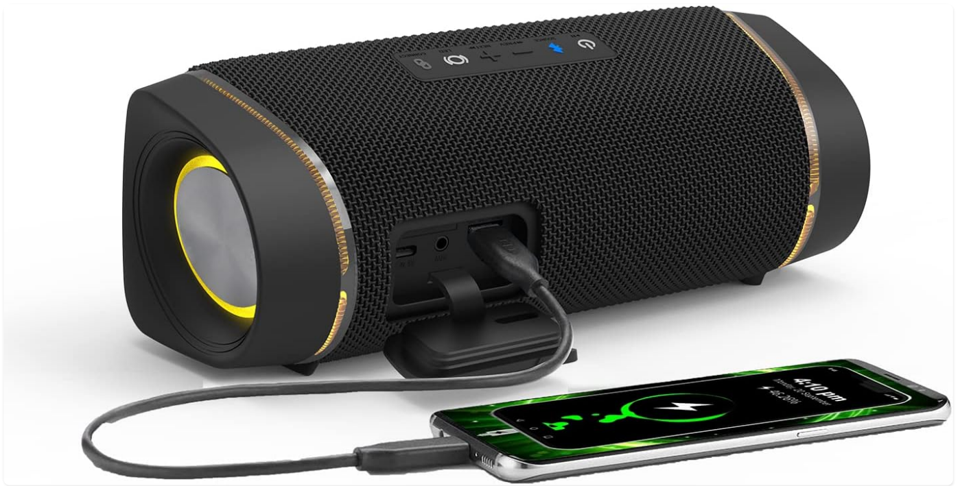
Figure 1: The speaker's rear panel with the protective flap open, showing the USB-C charging port and a smartphone connected for charging. The speaker's end panels glow with yellow light.
