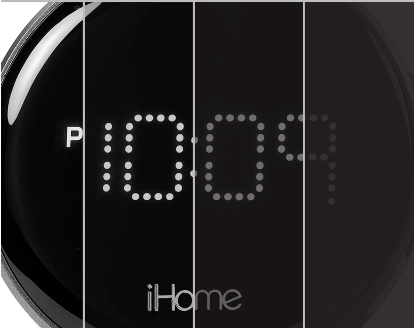
Figure 7: Auto-dimming display sensor in action.
