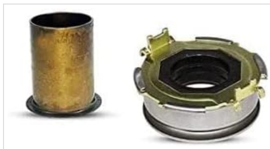
Figure 2.3: The clutch release bearing and bearing sleeve. The release bearing presses against the diaphragm spring of the pressure plate, while the sleeve guides the bearing's movement on the transmission input shaft.
