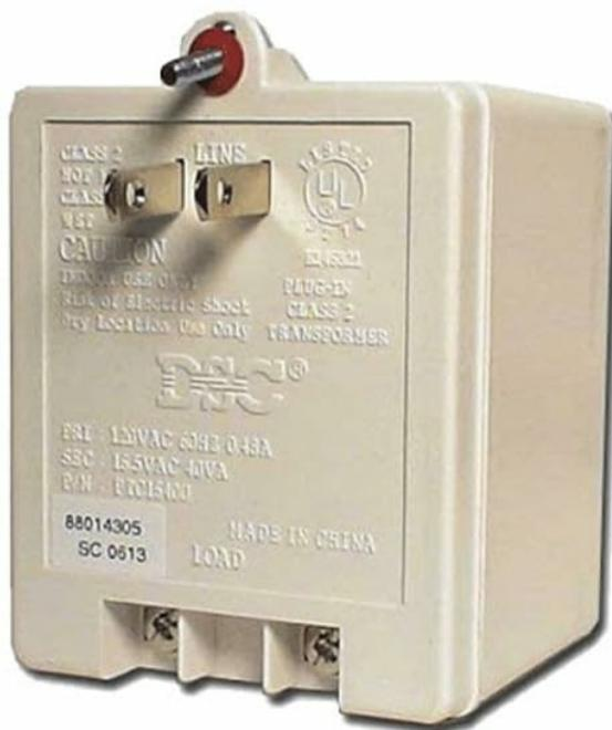
Figure 1: The DSC PTC1620U AC Transformer, showing its two-prong plug for wall outlets and the low-voltage screw terminals for connection to the alarm system. The label indicates input 120VAC 60Hz 0.43A and output 16.5VAC 20VA, and UL listing for dry locations.
