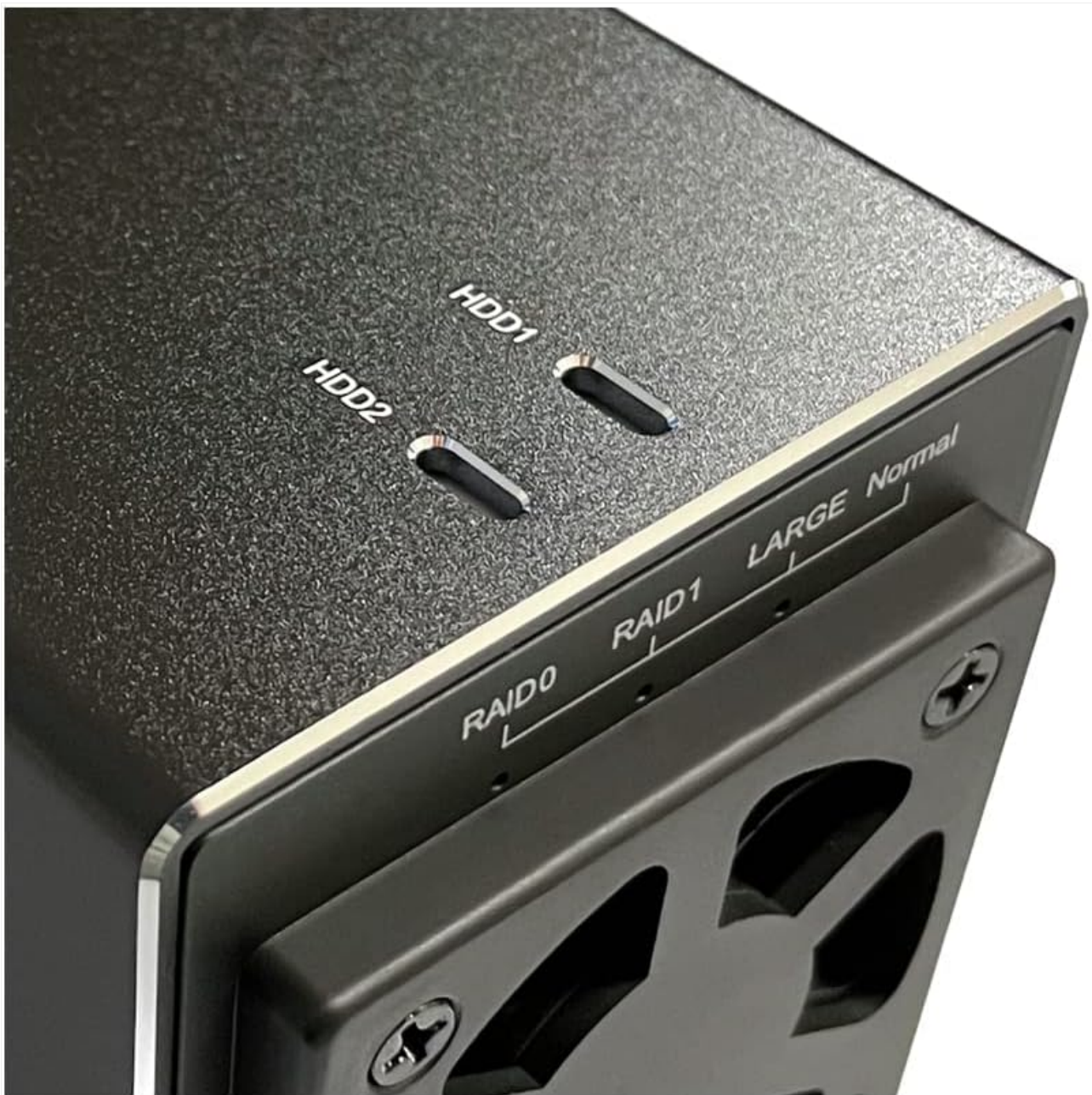
Figure 6: Top panel indicators for HDD activity and RAID mode labels.
