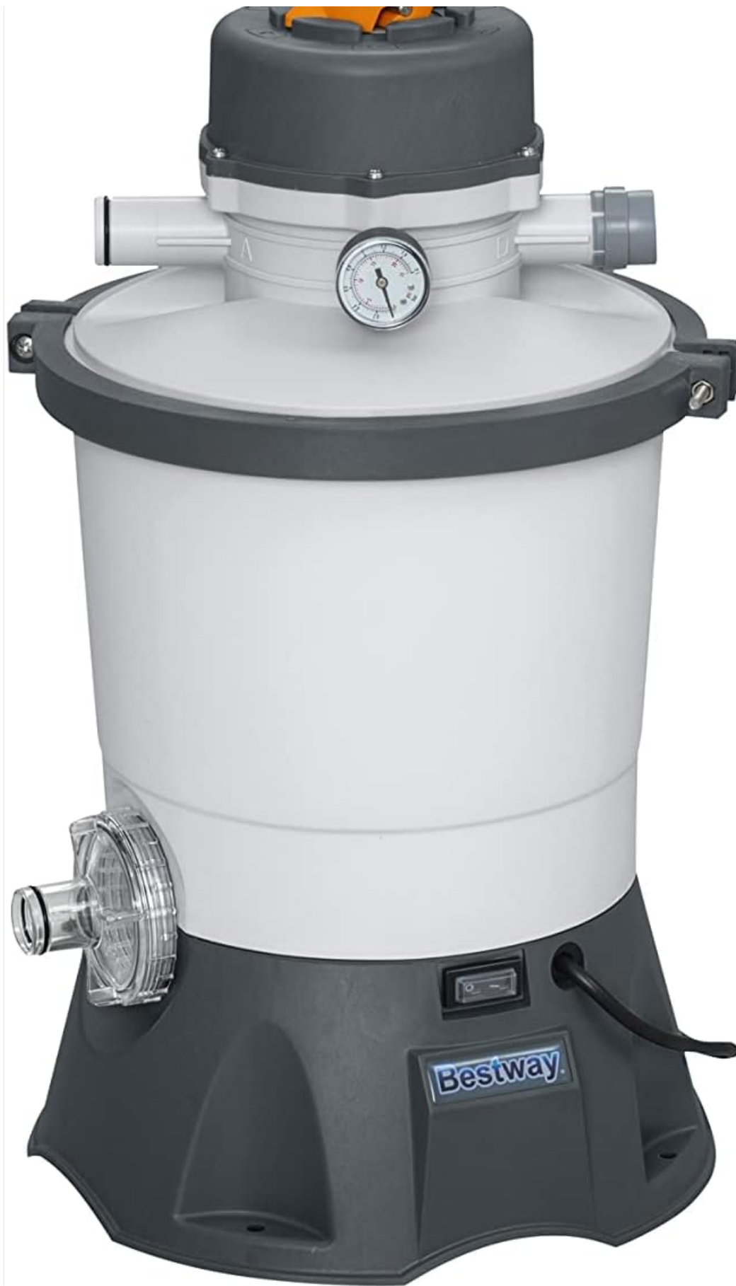
Figure 5: The pressure gauge indicates the filter's cleanliness. A rising pressure indicates a dirty filter.
