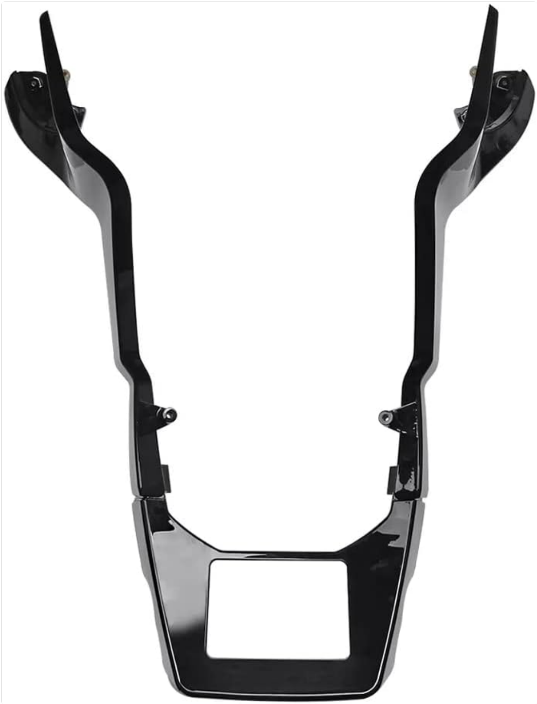
Figure 2: View of the fairing's internal structure and potential mounting points.
