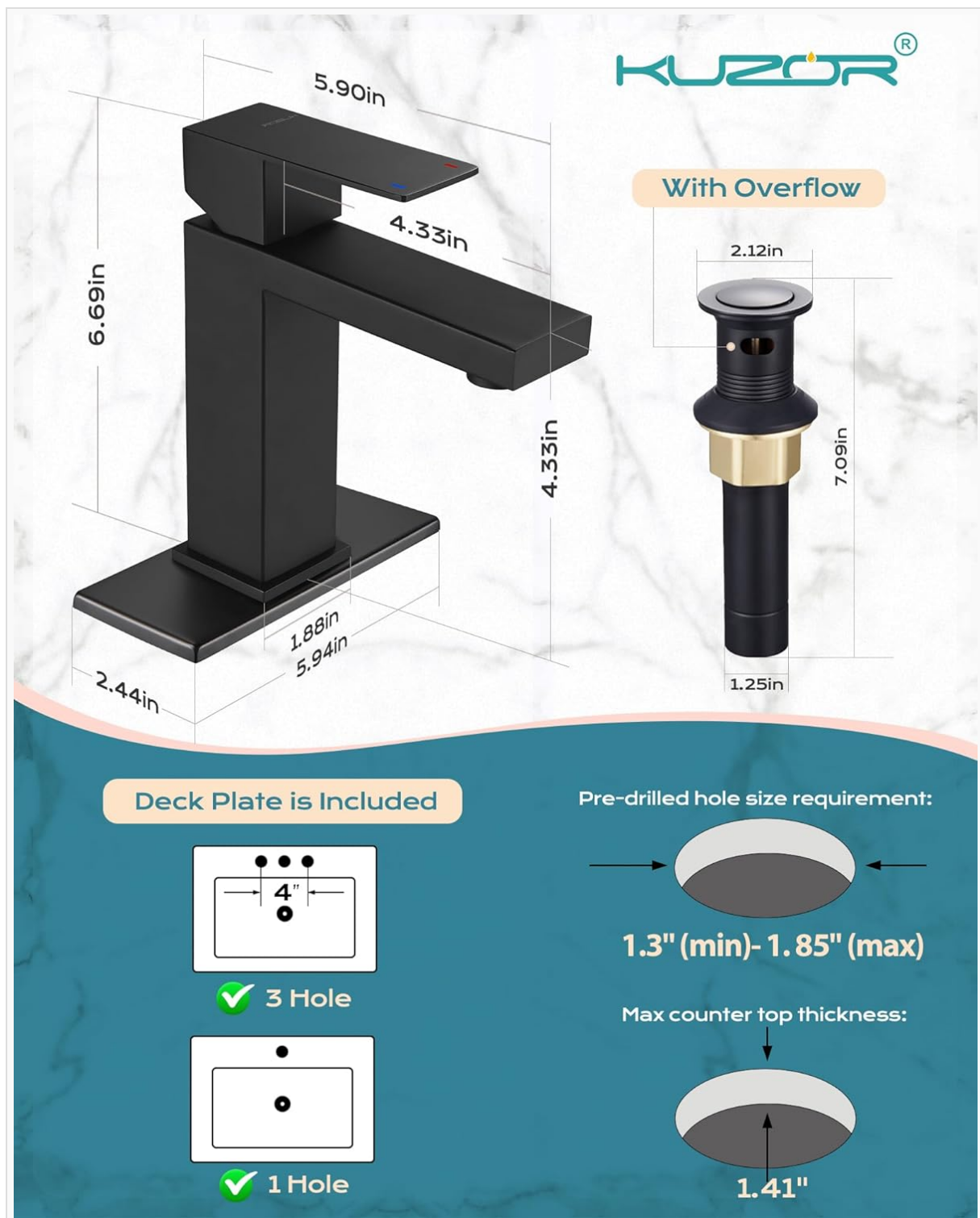
Figure 3.1: Detailed dimensions of the KUZOR faucet and pop-up drain, along with pre-drilled hole size requirements (1.3"-1.85" diameter) and maximum countertop thickness (1.41").
