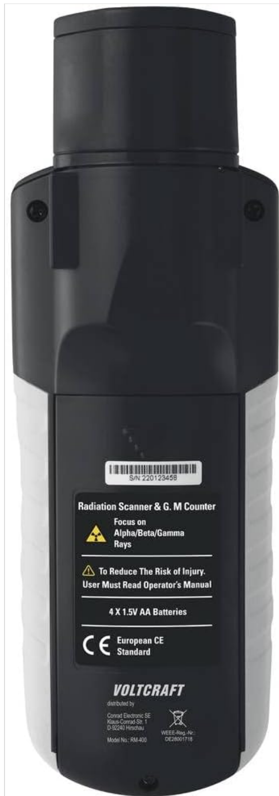
Figure 3.3: Rear view of the RM-400, indicating the battery compartment and safety warnings, including the requirement for 4x 1.5V AA batteries.
