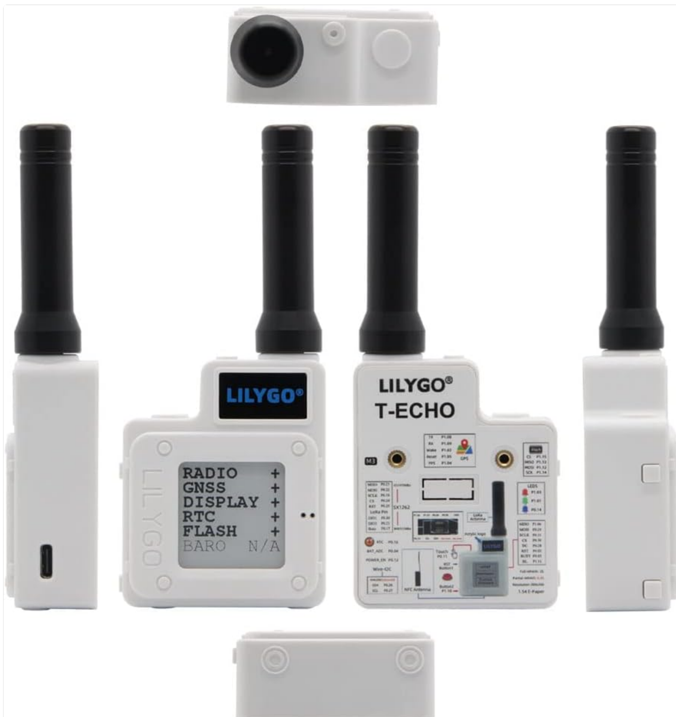
Figure 2.2: Various angles of the LILYGO T-Echo, showcasing its compact form factor and antenna.
